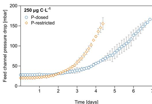
**Fig. 1.** Feed channel pressure drop [mbar] in time over the MFS for the P-restricted (<0.3 μg P·L<sup>-1</sup>) and the P-dosed (25 μg P·L<sup>-1</sup>) feed water conditions for a dosed high assimilable organic carbon concentration of 250 μg C·L<sup>-1</sup>. Fully independent duplicate experiments are shown. The MFSs were stopped and sampled for biofilm analysis once a feed channel pressure drop increase of 150 mbar was reached.
