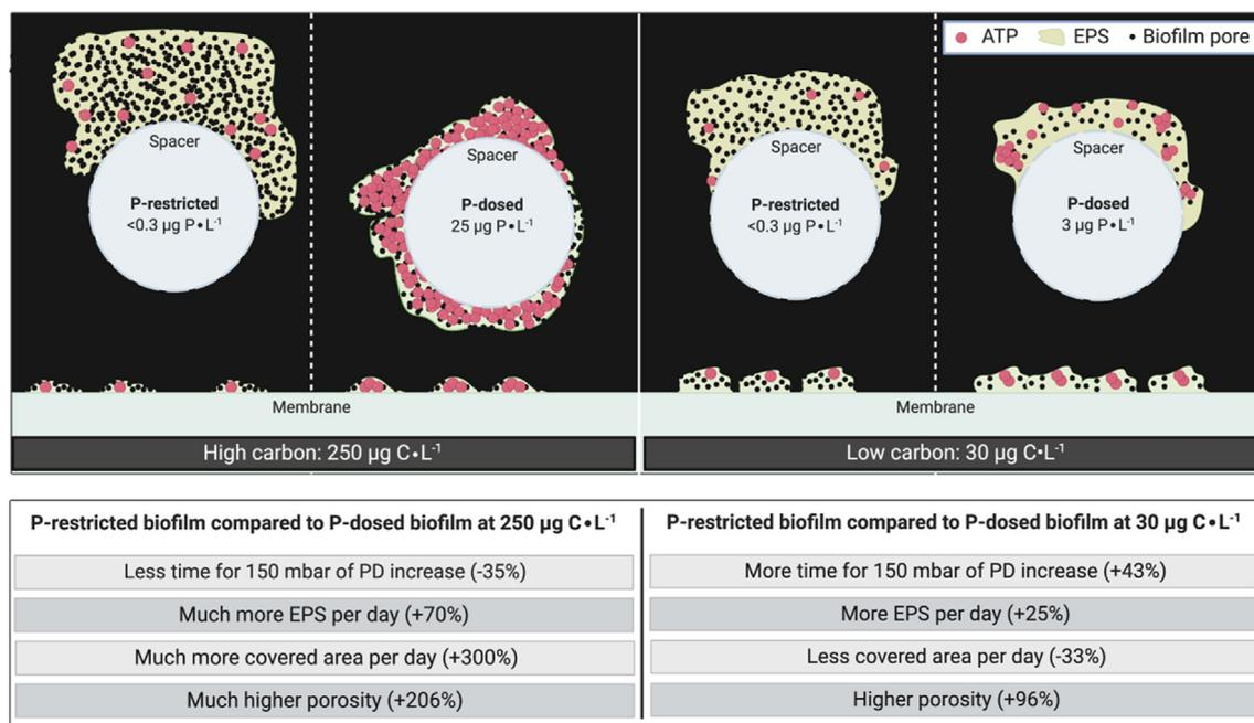
Fig. 7. Biofilm schematic for high ( $250 \mu\text{g C}\cdot\text{L}^{-1}$ ) and low ( $30 \mu\text{g C}\cdot\text{L}^{-1}$ ) carbon concentrations, at low phosphorus concentration (P-restricted  $<0.3 \mu\text{g P}\cdot\text{L}^{-1}$ ) in the feed water.
