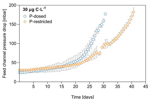
**Fig. 4.** Feed channel pressure drop [mbar] in time over the MFS for the P-restricted ( $<0.3 \mu\text{g P}\cdot\text{L}^{-1}$ ) and the P-dosed ( $3 \mu\text{g P}\cdot\text{L}^{-1}$ ) feed water conditions for a dosed assimilable organic carbon concentration of  $30 \mu\text{g C}\cdot\text{L}^{-1}$ . Fully independent duplicate experiments are shown. The MFSs were stopped and sampled for biofilm analysis once a feed channel pressure drop increase of 150 mbar was reached.
