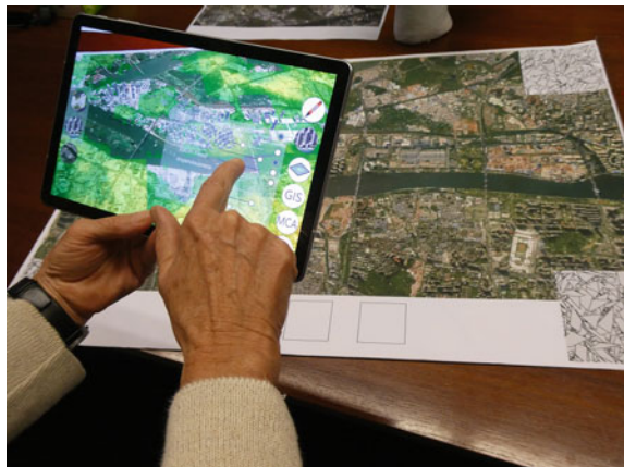
Fig. 1.9 Augmented reality (AR) interface that allows for enriching GIS maps with overlays of design alternatives while running a dynamic multi-criteria analysis. Photo Eckart Lange
