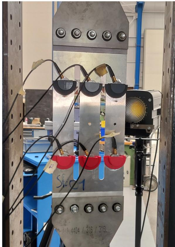
Figure 4.8: Example of the fixation of the AE sensors to one of the specimens tested.
