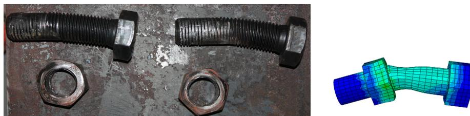
Fig.9.12. Stress state at the end of test for bolts in top tensile row of 1-2 P (S690 12mm) after cooling down from fire.
