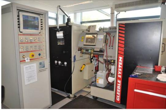
Fig.4.1. Test device-Gleeble 3800 system.
