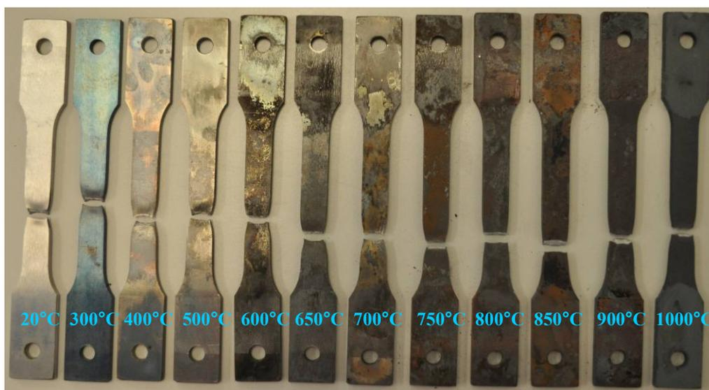
Fig.5.16. Failure mode of S960 tensile specimens after exposure to various elevated temperatures.
