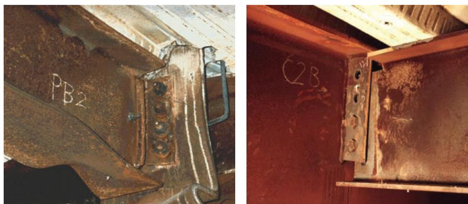
Fig.2.6. Failure modes of flexible end-plate and fin-plate joints in Cardington fire tests [37].
