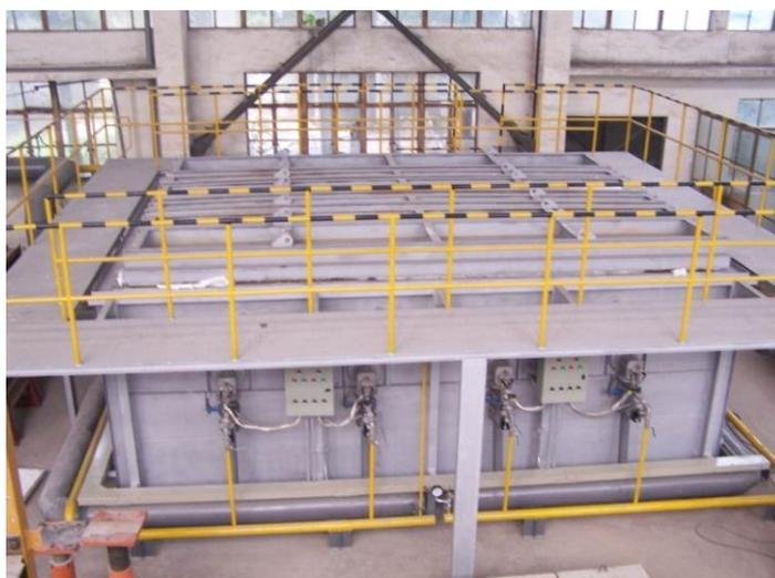
Fig. 6.2. Fire test furnace.
