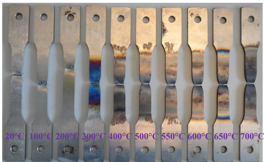
Fig.4.33. Failure mode of S960 specimens at elevated temperatures under steady state condition.
