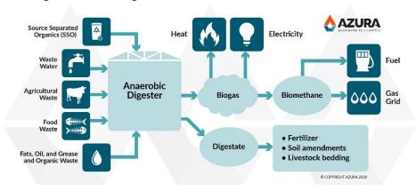
An anaerobic digester is a biological system used to break down organic materials, such as food waste, agricultural residues, and sewage sludge, in the absence of oxygen (anaerobic conditions). Its primary function is to convert these organic materials into biogas and nutrient-rich effluent through a microbial fermentation process. Here's how it works:
