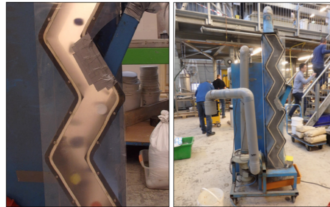
figure 7.6.2, particles rotating in the zigzag vortexes
