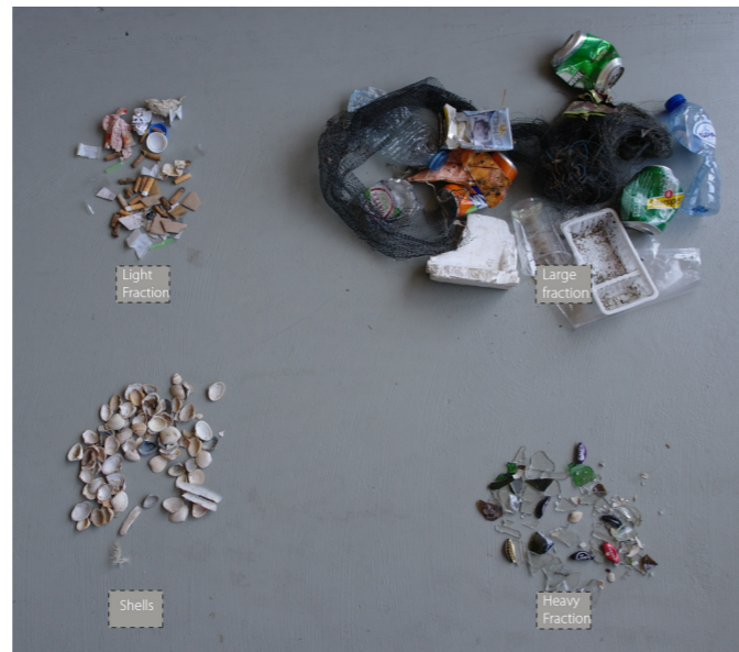
Figure 9.2.2, four fractions into which the prototype separates
