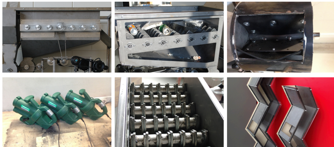
figure 9.2.1, F.L.T.R, electrical drive, discscreen, rotary valve, blowers, discscreen mesh, zigzag channels
