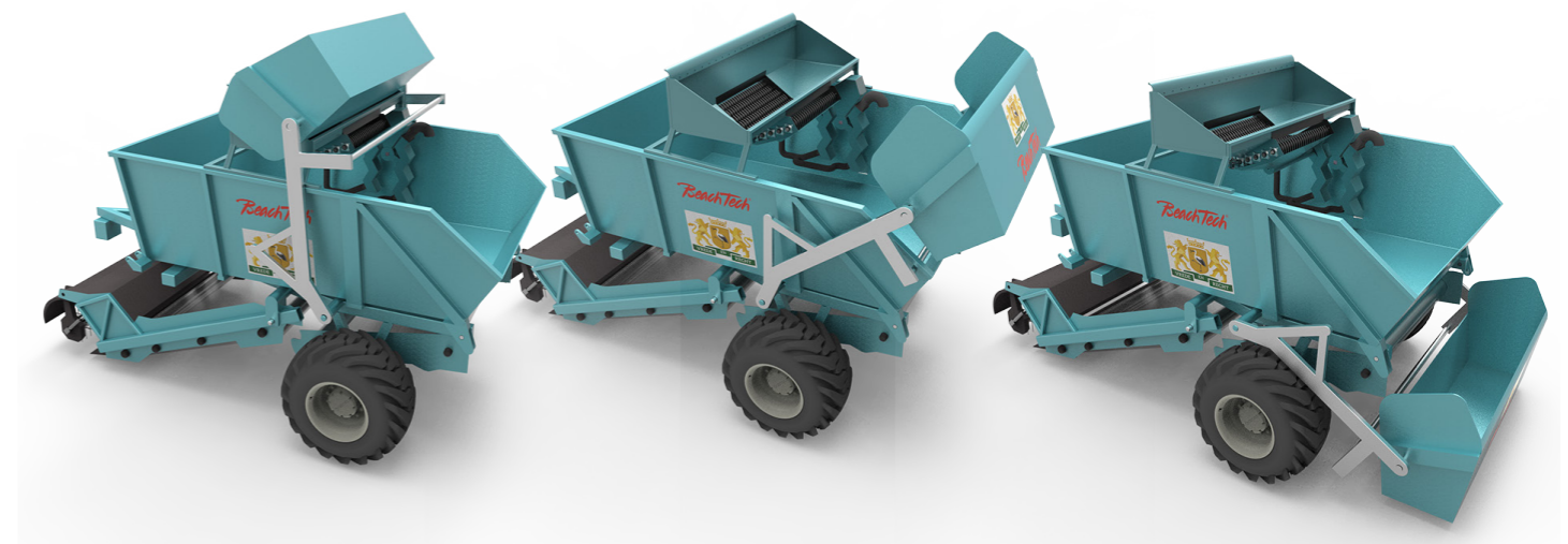
figure 9.3.2, top, material flow through the beach cleaner with the shell saver, bottom, filling the hopper of the shell saver with collected material
