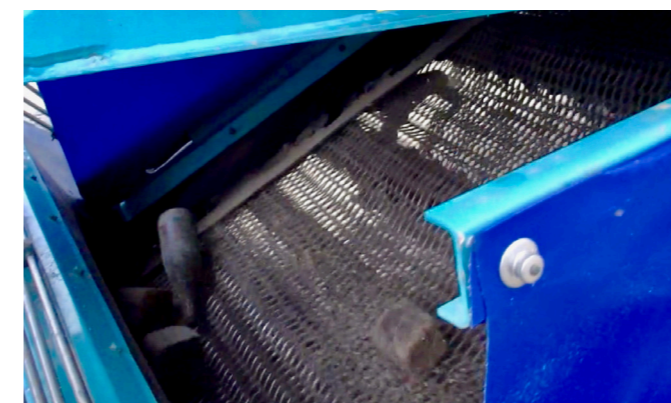
figure 4.4.6, stones inside the beach cleaner brake glass
