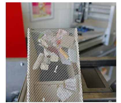
Figure 9.2.6, "lights" get stuck to the air exit screen.
