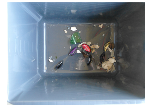
Figure 9.2.4, bottle caps and thin pieces of glass in the shell container
