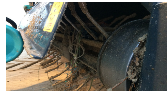
figure 4.4.5, ropes get stuck in the raking unit.
