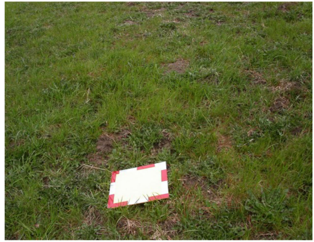
(b) Reasonable: at most 5 spots with a diameter < 0.2 m where vegetation is gone.
