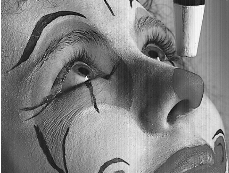
Figure 4-23: DCS simulation under the same parameters as Figure 4-22, but with 2% column FPN in the image
