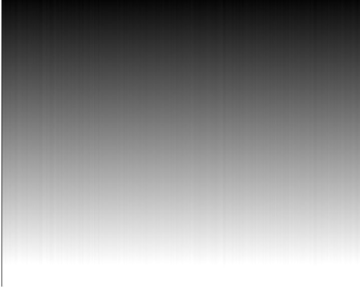
Figure 5-10: image acquired using a test input voltage increasing each line time, without circuit auto-zero
