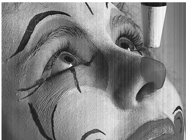
Figure 4-20: Sample image with 3% Gaussian column FPN. DCS is simulated on the left half of the image using a 5x5 unit switching cell
