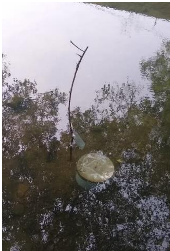
Figure 5.13: The bag is connected to the bucket through the hose. The bag is completely underwater.
