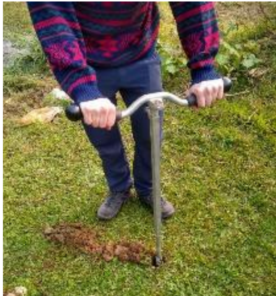
Figure 8.6: Drilling a borehole using the auger and handle.
