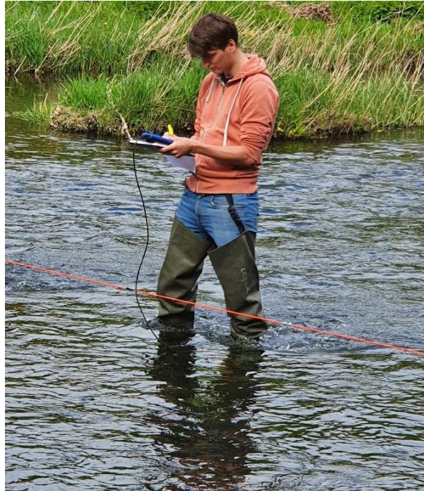
Figure 4.18: A person measuring the EC in the middle of the stream. In one hand, the observer holds the clipboard with the record sheet. Firmly attached to the clipboard is the EC meter, with the probe hanging into the water. The probe is completely submerged, but not touching the bottom of the river. In his other hand, the observer holds the pen and writes down the measured EC.
