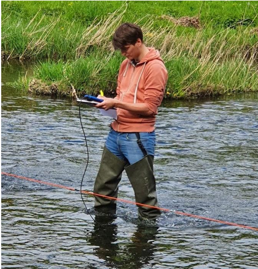
Figure 4.13: A person measuring the EC in the middle of the stream. In one hand, the observer holds the clipboard with the record sheet. Firmly attached to the clipboard is the EC meter, with the probe hanging into the water. The probe is completely submerged, but not touching the bottom of the river. In his other hand, the observer holds the pen and writes down the measured EC.
