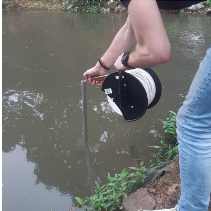
Figure 5.7: Measuring the water level inside the piezometer
