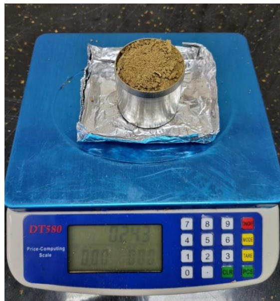
Figure 10.10: Weighing the soil sample after it has been fully saturated.
