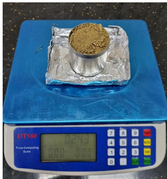
Figure 10.12: Weighing the sample after it has dried in the oven.
