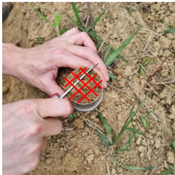
Figure 10.5: Carefully cutting a grid into the soil that is sticking out above the top of the ring.
