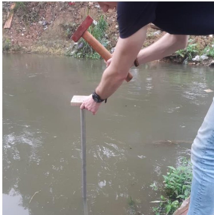
Figure 5.6: Hammering the piezometer into the riverbed
