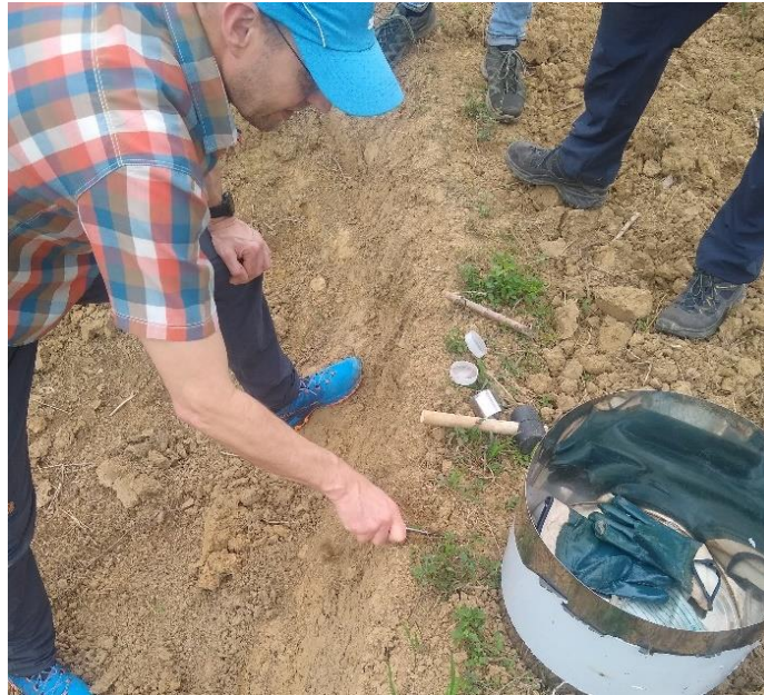
Figure 10.2: Removing the topsoil layer.
