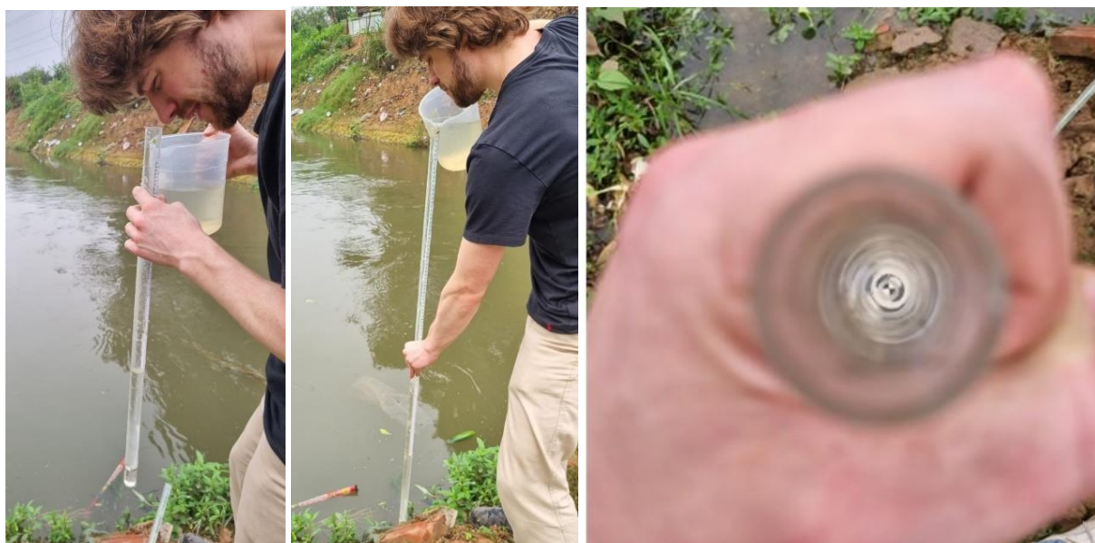
Figure 6.5: Left: using the bottom section of the transparency tube. Middle: using the bottom and top sections. Right: Secchi tube visible through the water
