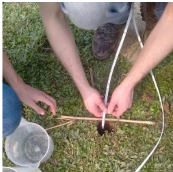
Figure 8.8: Measuring the water depth using a piece of wood, so that the reference level is always constant
