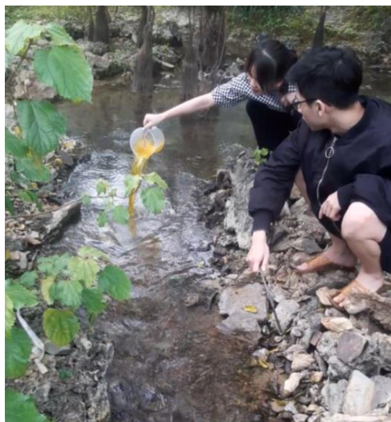
Figure 4.16: Injecting coloring agent into the stream to see if it has sufficient turbulent mixing. Here, a yellow coloring agent is used. Red or green are often more suitable.
