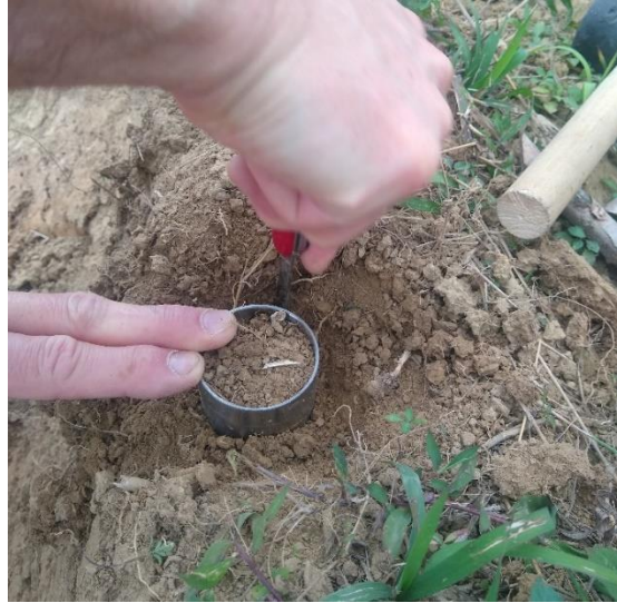
Figure 10.4: Removing some of the soil around the ring.
