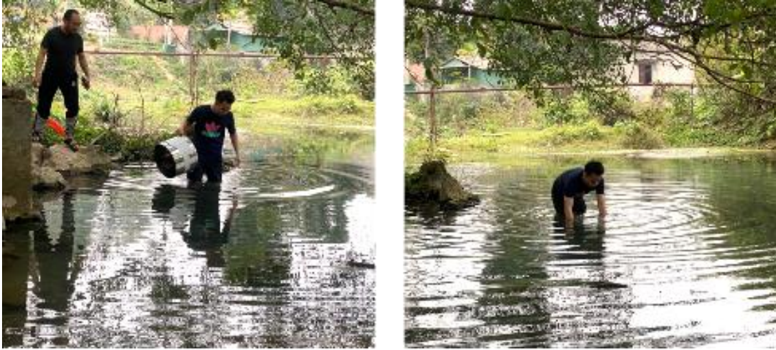
Figure 5.10: Installing the seepage meter into the bottom of the pond.
