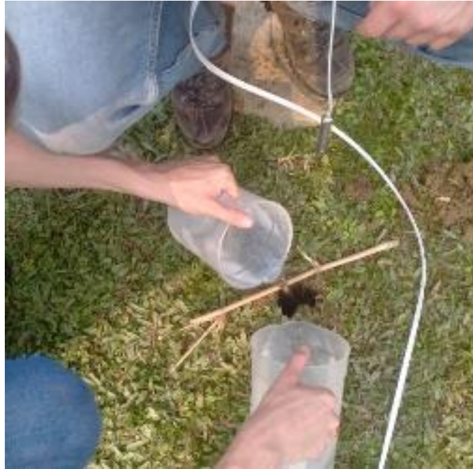
Figure 8.9: Filling the hole with water.
