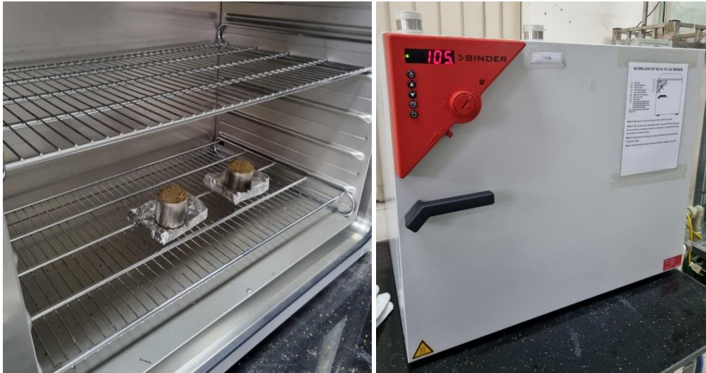
Figure 10.11: Putting the saturated soil samples in a 105 °C oven to dry for 24 hours.
