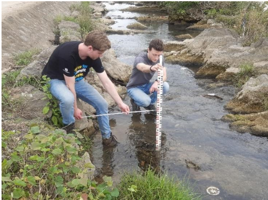
Figure 4.11: Measuring the water depth
