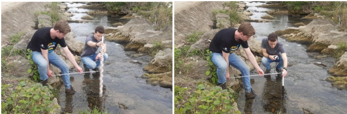
Figure 2.5: Measuring the depth of a segment, followed by measuring the flow velocity of a segment
