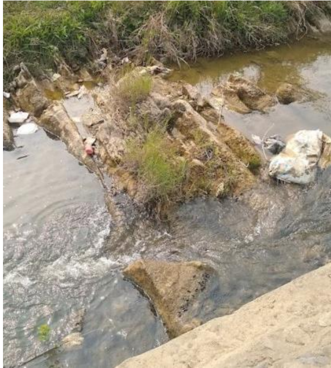
Figure 4.15: A suitable injection point, where the water is quite turbulent with some rapids, and all the water flows through a narrow cross-section
