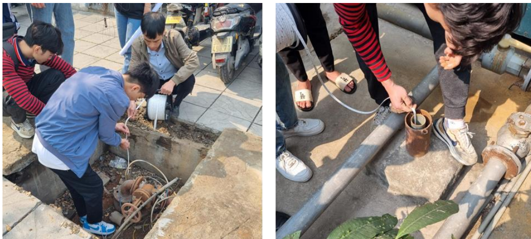
Figure 7.7: Doing a manual measurement of the water level inside the pumping well (left) and observation well (right)
