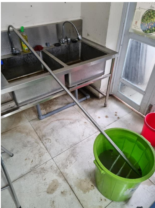
Figure 5.8: Cleaning the portable piezometer using water pressure
