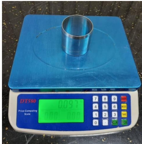
Figure 10.13: Weighing the ring.
