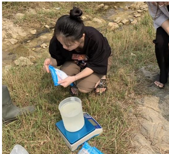
Figure 4.12: Dissolving salt into a bucket. Notice how the salt is carefully weighed.
