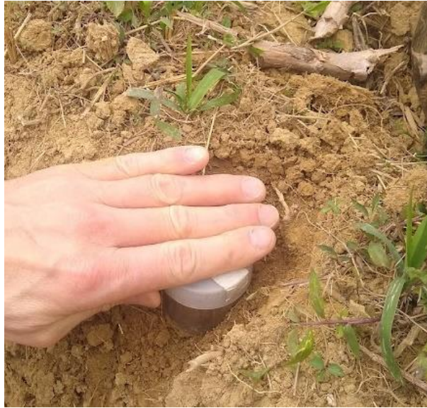
Figure 10.6: Putting the lid on the ring, after having removed excess soil.
