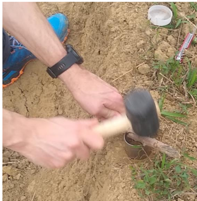
Figure 10.3: Hammering the ring into the soil.
