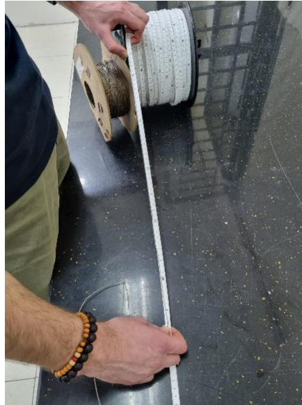
Figure 7.8: Getting the right length of metal string.
