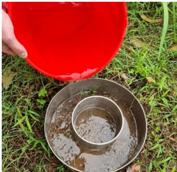
Figure 9.5: Refilling the outer ring of water.
