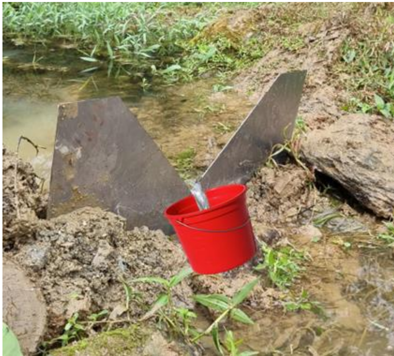
Figure 3.10: Measuring the discharge using the volumetric method. This method is sometimes called the bucket-and-stopwatch method.
