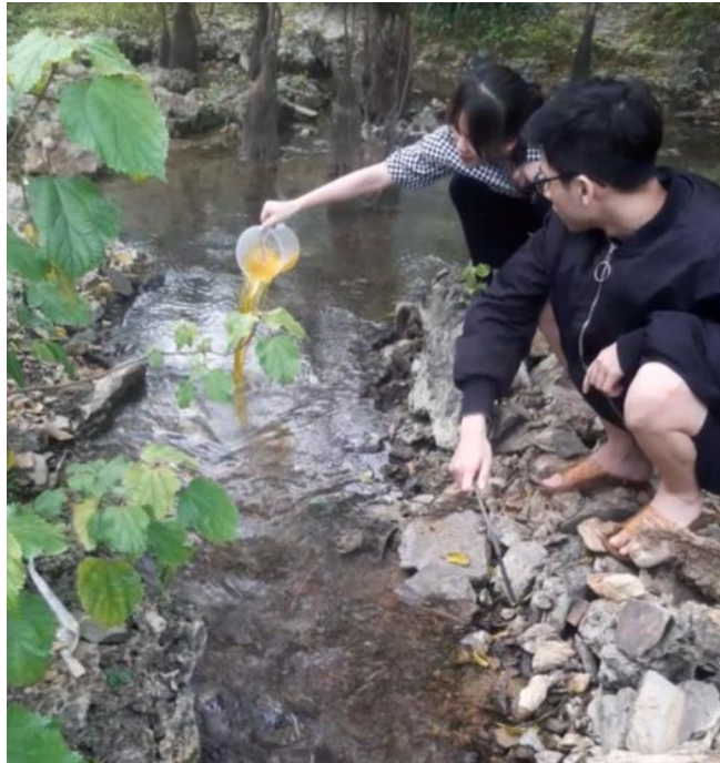
Figure 4.9: Injecting coloring agent into the stream to see if it has sufficient turbulent mixing. Here, a yellow coloring agent is used. Red or green are often more suitable.
