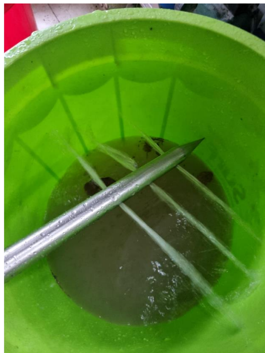
Figure 5.8: Cleaning the portable piezometer using water pressure
