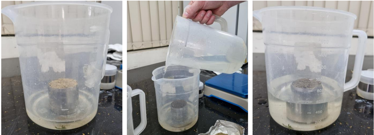
Figure 10.9: Saturating the soil sample from below.
