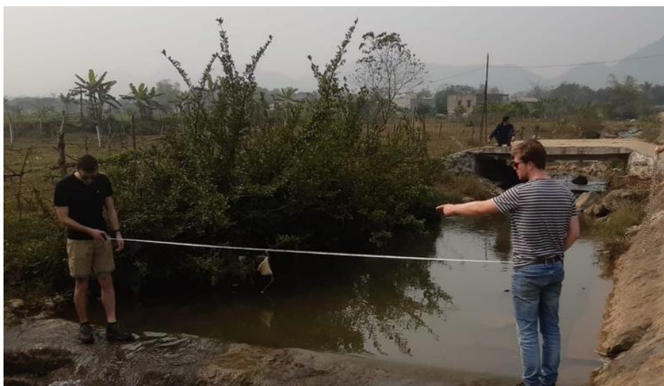
Figure 4.10: Spanning a measuring tape across the stream, orthogonal to the direction of flow
