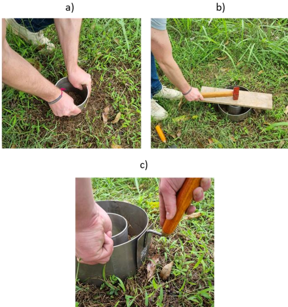
Figure 9.2: Inserting the rings into the ground using various methods.
