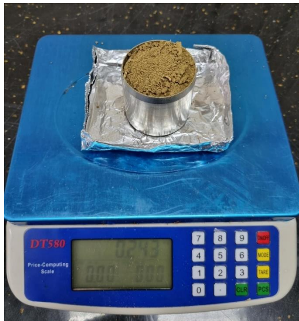
Figure 10.8: Weighing the soil sample.
