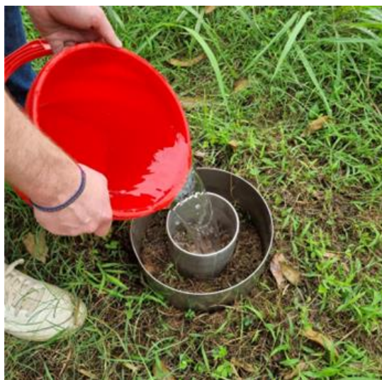
Figure 9.3: Filling the rings with water.
