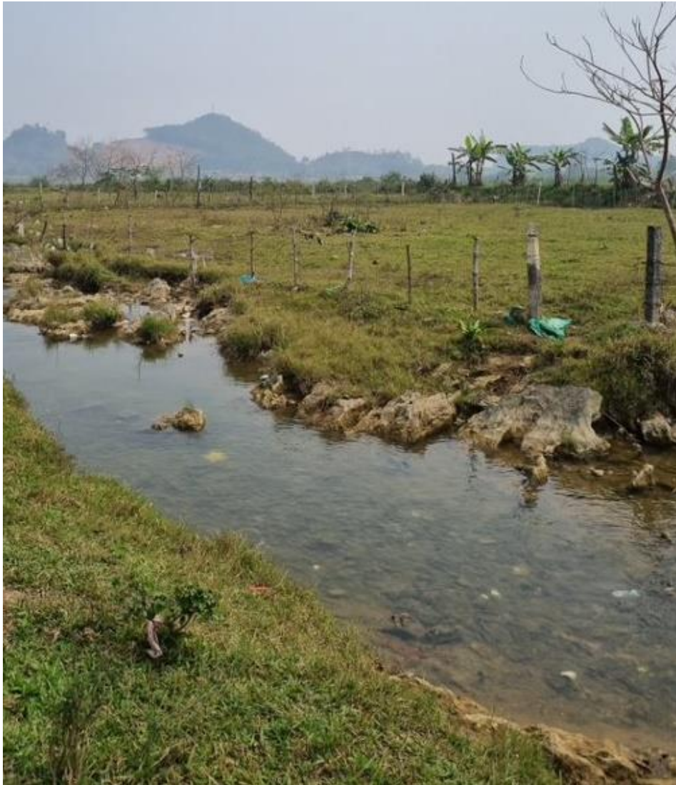
Figure 4.8: A suitable downstream section, with more or less a constant cross-section and no major turns
