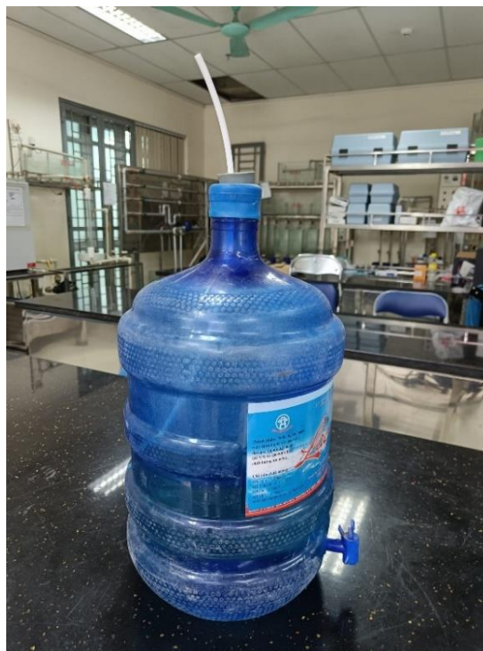
Figure 4.3: A Mariotte bottle, which discharges at a constant rate
