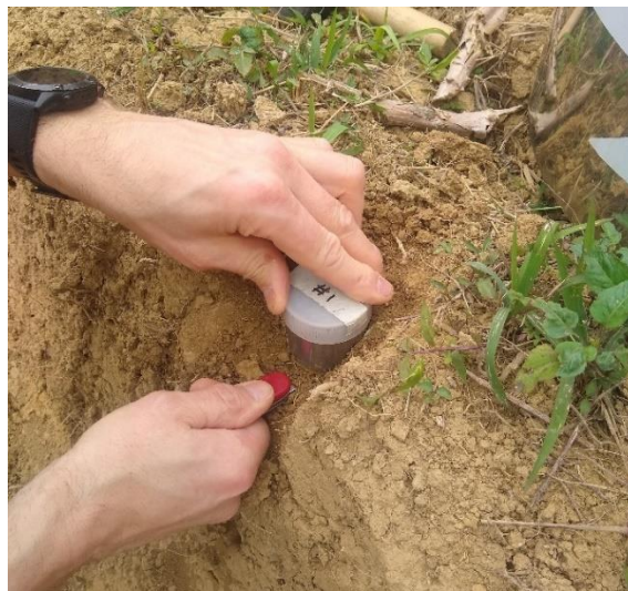
Figure 10.7: Cutting horizontally below the ring.
