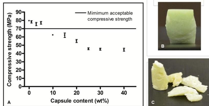
Figure 1: (A) Relationship between capsule content and the ultimate compressive strength of bone cement (average  $\pm$  SEM,  $n=3$  with 5 replicates per group). Photographs of samples containing (B) 0 wt% and (C) 40 wt% capsules post-compression testing.
