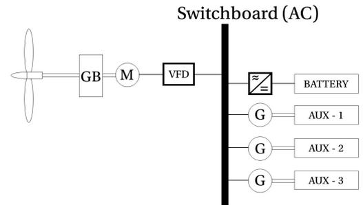
Figure 5.17: An electric powertrain configuration powered by an ICE and a battery with an alternative current switchboard
