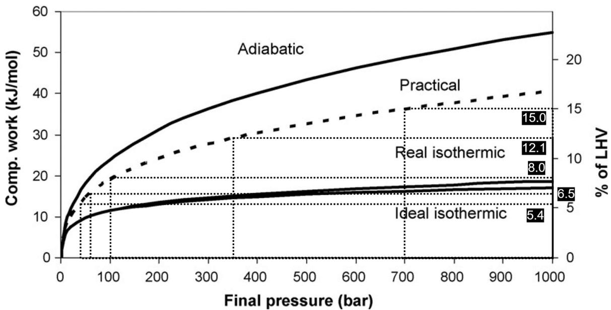
Figure 2.2: The energy needed for the compression of hydrogen[31]
