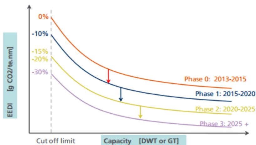
Figure C.1: The energy efficiency design index of the IMO[152]
