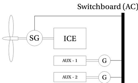
Figure 5.11: Two stroke engine configuration with two auxiliary engines
