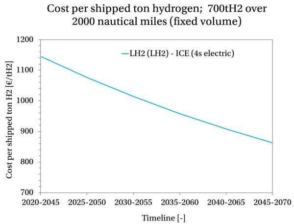
Figure 7.7: Cost per shipped ton hydrogen, when fixing the size of the ship
