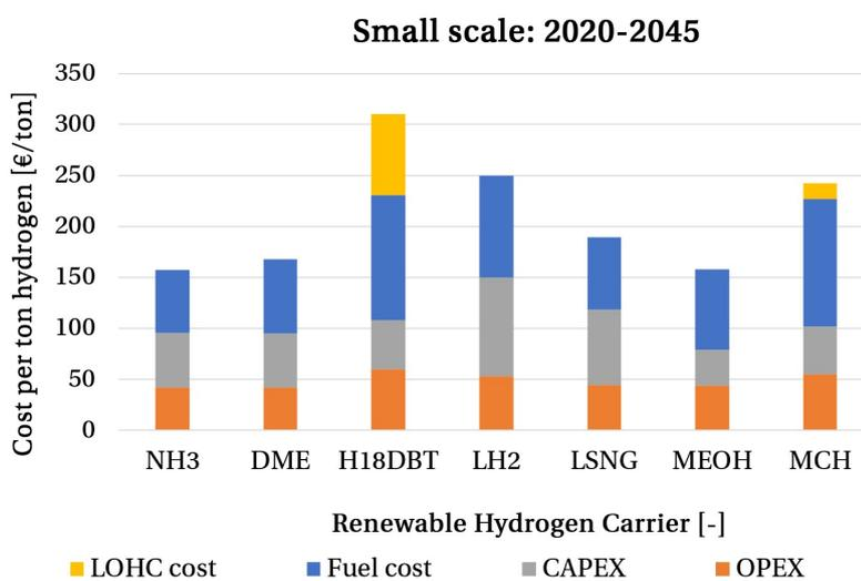
Figure 3.7: Cost per ton hydrogen delivered for the small scale case based on RHC prices in the short term
