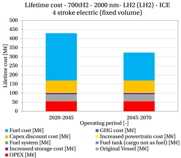
Figure 7.9: Total cost over lifetime, when fixing ship size
