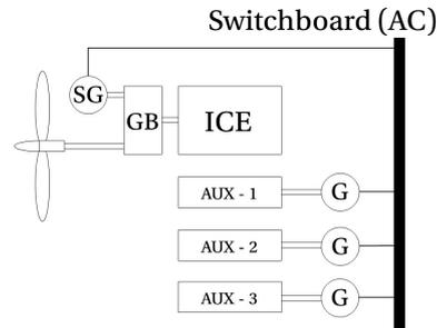
Figure 5.13: Four stroke engine powertrain configuration
