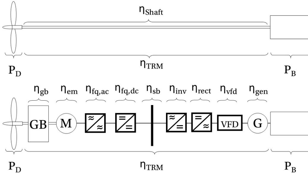
Figure 5.10: Different powertrain configurations can affect the efficiency of the transmission from the prime mover to the propeller
