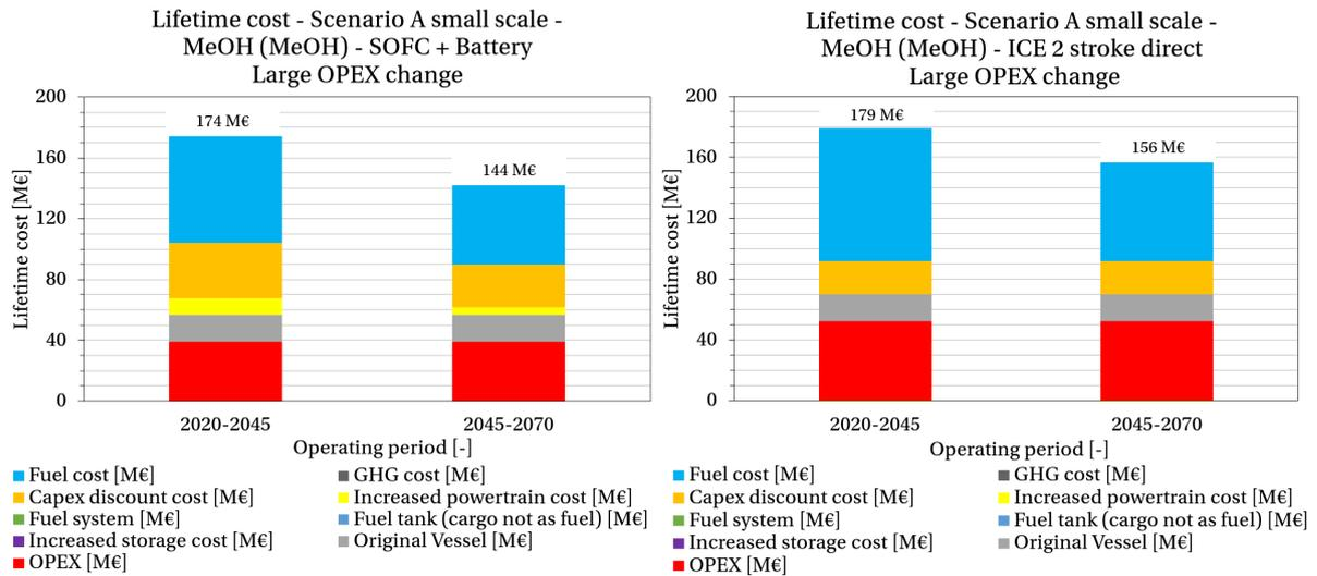
Figure 7.12: Total cost over lifetime, of two different powertrain configurations (left: SOFC + Battery, right: ICE 2 stroke) on a methanol carrier with a large reduction of OPEX for the SOFC + Battery powertrain
