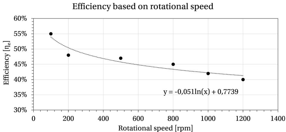
Figure 5.6: The effect of the rotational speed on the efficiency of the engine [106]
