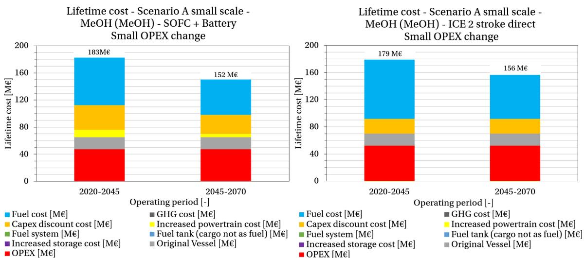
Figure 7.11: Total cost over lifetime, of two different powertrain configurations (left: SOFC + Battery, right: ICE 2 stroke) on a methanol carrier with a small reduction of OPEX for the SOFC + Battery powertrain
