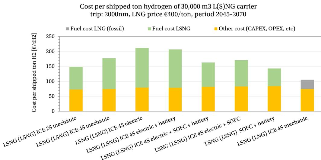
Figure 7.3: Cost of transported hydrogen per ship in a typical LNG 30,000 m<sup>3</sup> carrier operating between 2045 and 2070
