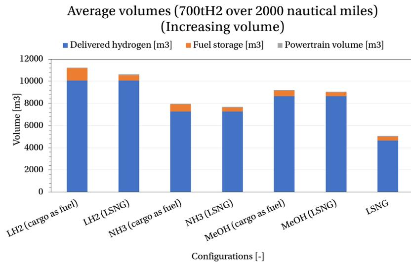
Figure 7.4: Average volume distribution of the different powertrain configurations for a trip over 2000 nautical miles with a design based on the transport of 700 ton hydrogen
