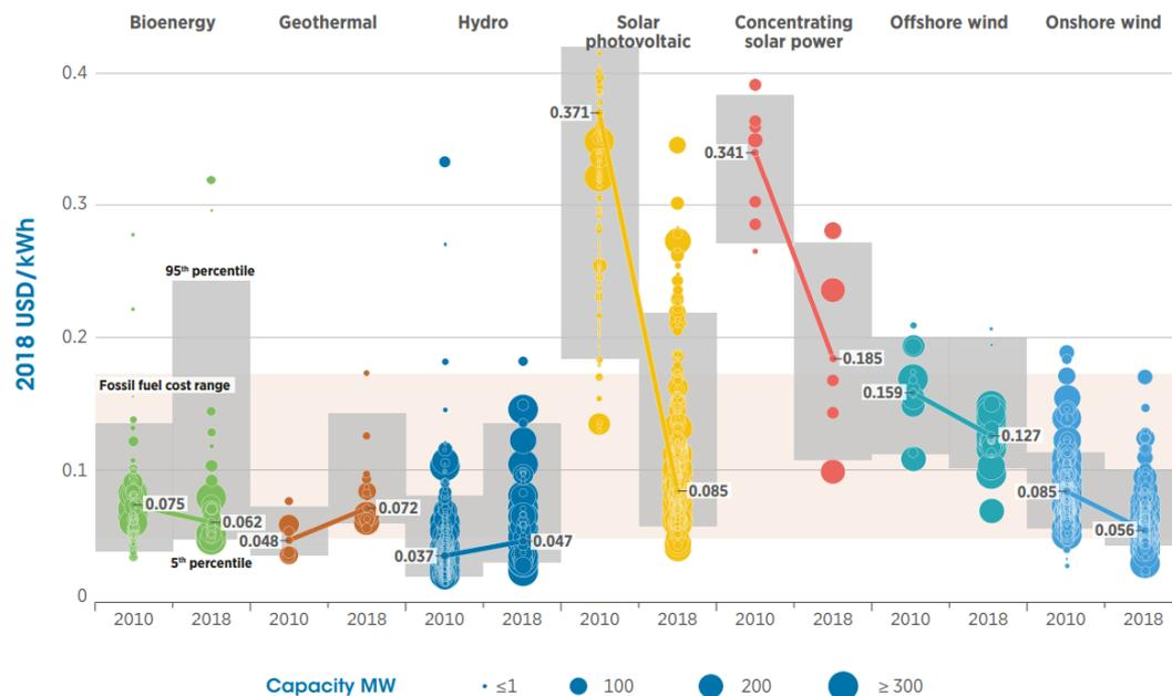
Figure 1.1: Global global weighted-average levelised cost of electricity of utility-scale renewable power generation technologies, 2010–2018 [6]
