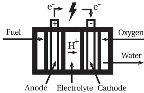
Figure 5.7: The working principle of a PEMFC
