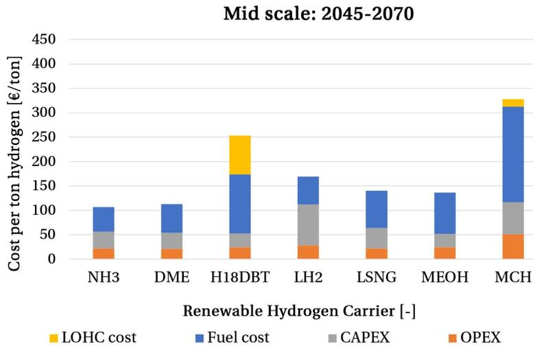
Figure 3.10: Cost per ton hydrogen delivered for the mid scale case based on RHC prices in the long term
