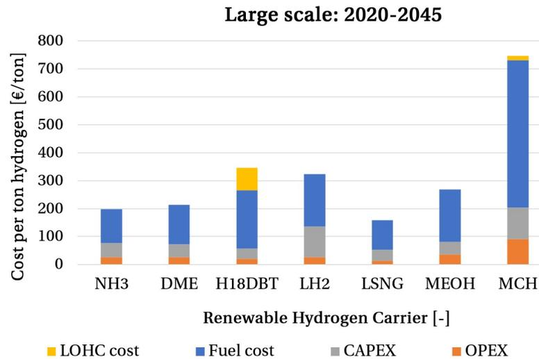
Figure 3.11: Cost per ton hydrogen delivered for the large scale case based on RHC prices in the short term
