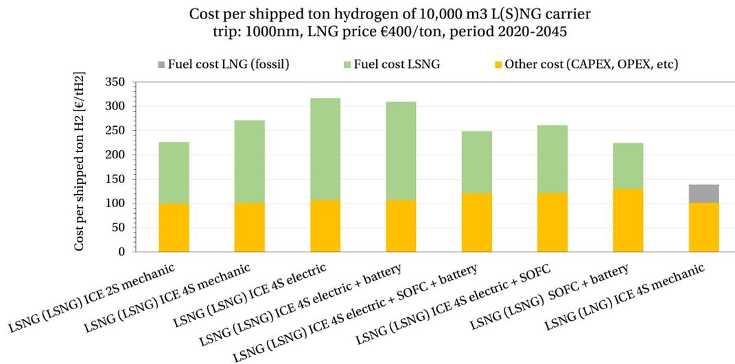
Figure 7.1: Cost of transported hydrogen per ship in a typical LNG 10,000 m<sup>3</sup> carrier operating between 2020 and 2045
