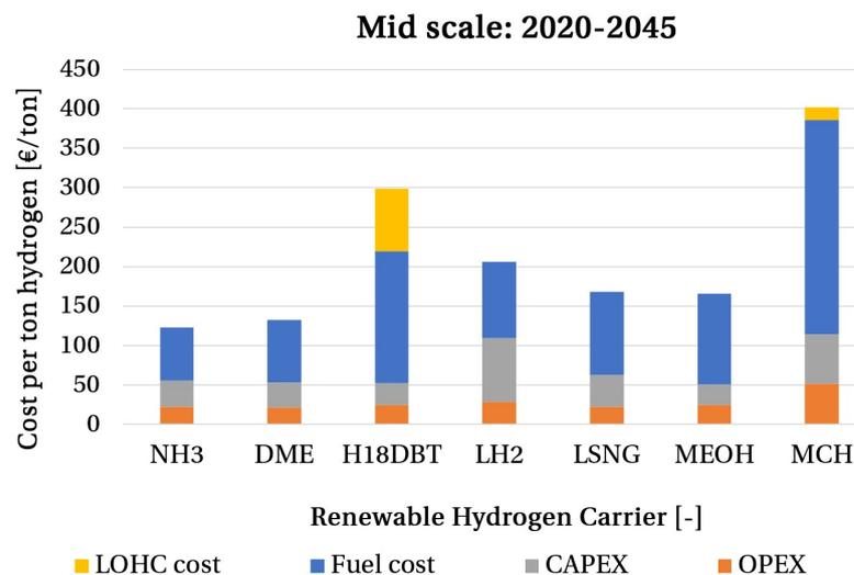
Figure 3.9: Cost per ton hydrogen delivered for the mid scale case based on RHC prices in the short term
