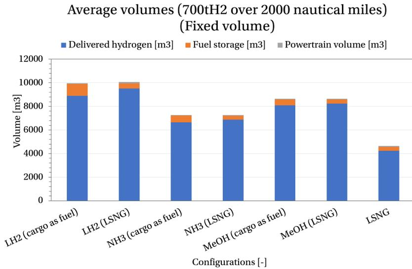
Figure 7.5: Average volume distribution of the different powertrain configurations for a trip over 2000 nautical miles with a design based on the transport of 700 ton hydrogen. This is for a fixed cargo volume
