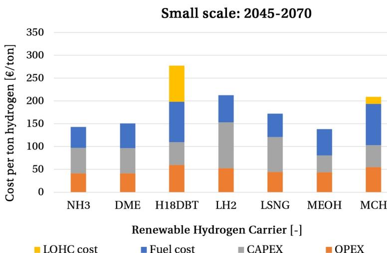
Figure 3.8: Cost per ton hydrogen delivered for the small scale case based on RHC prices in the long term
