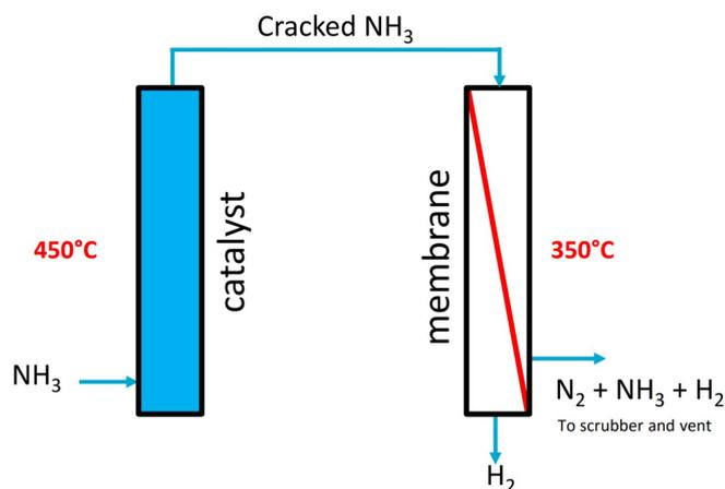
Figure 5.20: Ammonia reformer developed by CSIRO[130]
