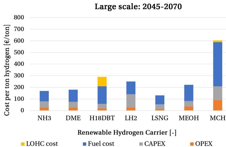
Figure 3.12: Cost per ton hydrogen delivered for the large scale case based on RHC prices in the long term
