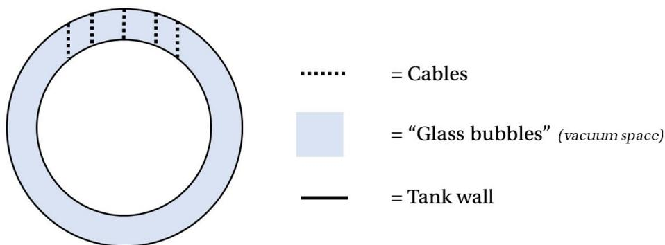
Figure 5.3: Storage tank design from NASA for liquefied hydrogen (LH<sub>2</sub>)
