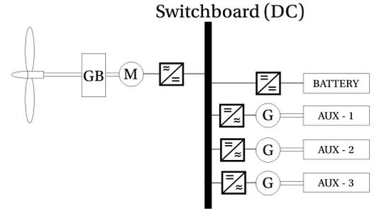
Figure 5.15: An electric powertrain configuration powered by an ICE and a battery with a direct current switchboard
