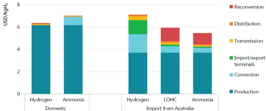
Figure 1.5: Cost of delivering hydrogen or ammonia produced via electrolysis, domestically, or from Australia to an industrial customer in Japan in 2030 [8]
