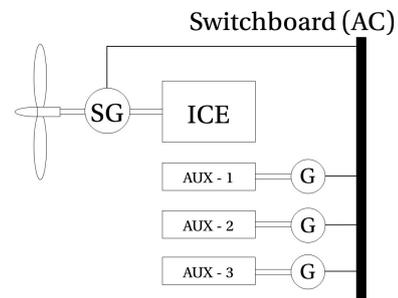
Figure 5.12: Two stroke engine configuration with three auxiliary engines
