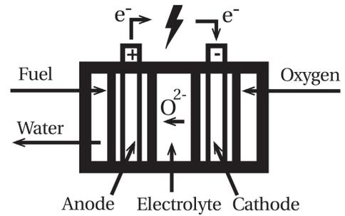
Figure 5.8: The working principle of a SOFC
