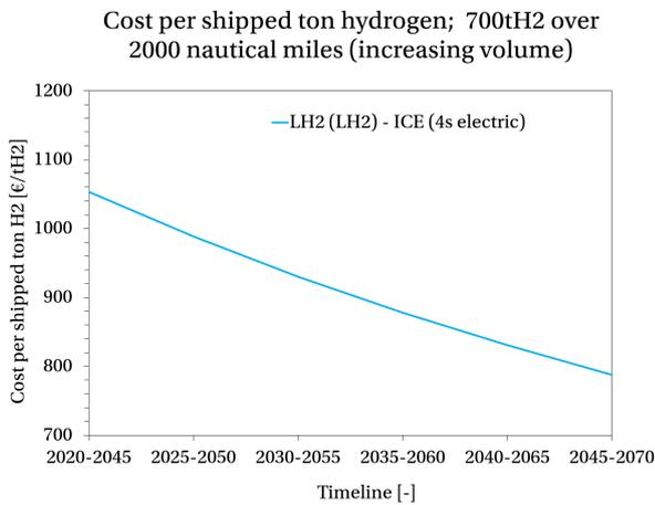
Figure 7.6: Cost per shipped ton hydrogen, when increasing ship size
