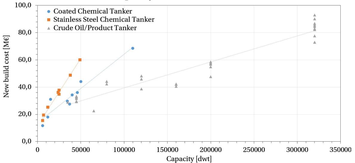
Figure 3.3: New build cost of chemical, crude oil and product tankers
