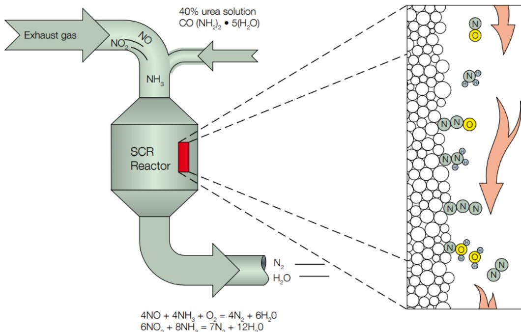
Figure 5.21: Working principle of an selective catalytic reduction (SCR) reactor[132]
