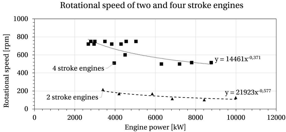
Figure 5.5: The rotational speed of combustion engines against the engine power based on database of Anthony Veder
