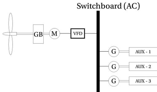
Figure 5.16: An electric powertrain configuration powered by an ICE with an alternative current switchboard
