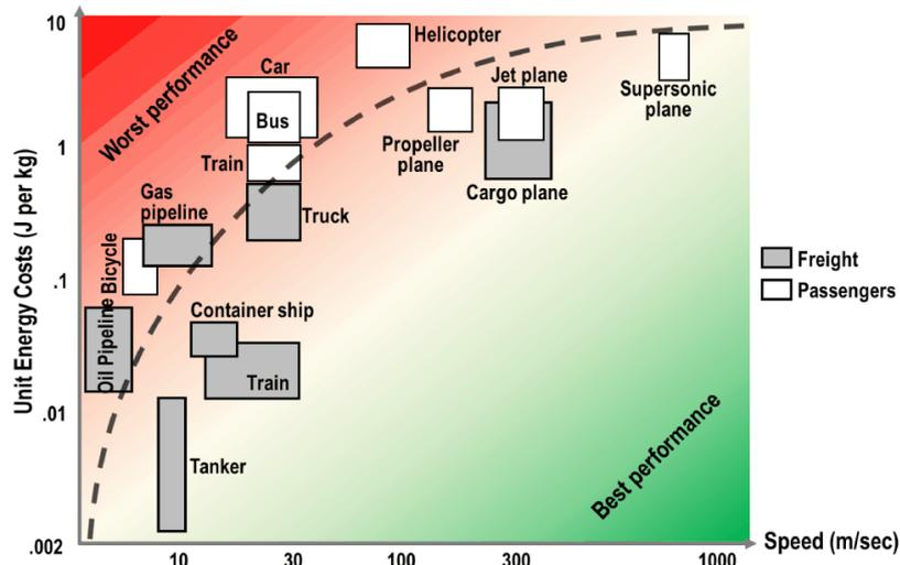
Figure 1.3: Energy efficiency of different forms of transportation [10]
