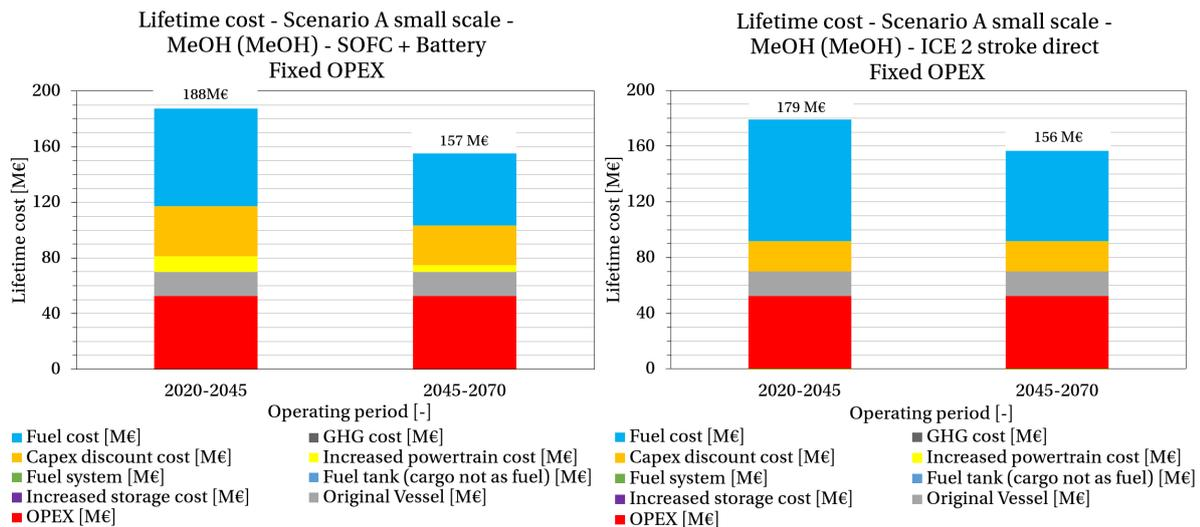
Figure 7.10: Total cost over lifetime, of two different powertrain configurations (left: SOFC + Battery, right: ICE 2 stroke) on a methanol carrier with a fixed OPEX
