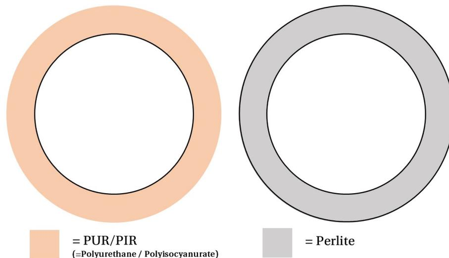
Figure 5.2: The storage types of LSNG considered in this thesis, on the left the single wall storage tank and on the right the double wall storage tank
