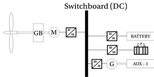
Figure 5.19: An electric powertrain configuration powered by an ICE, a battery and a fuel cell with direct current switchboard
