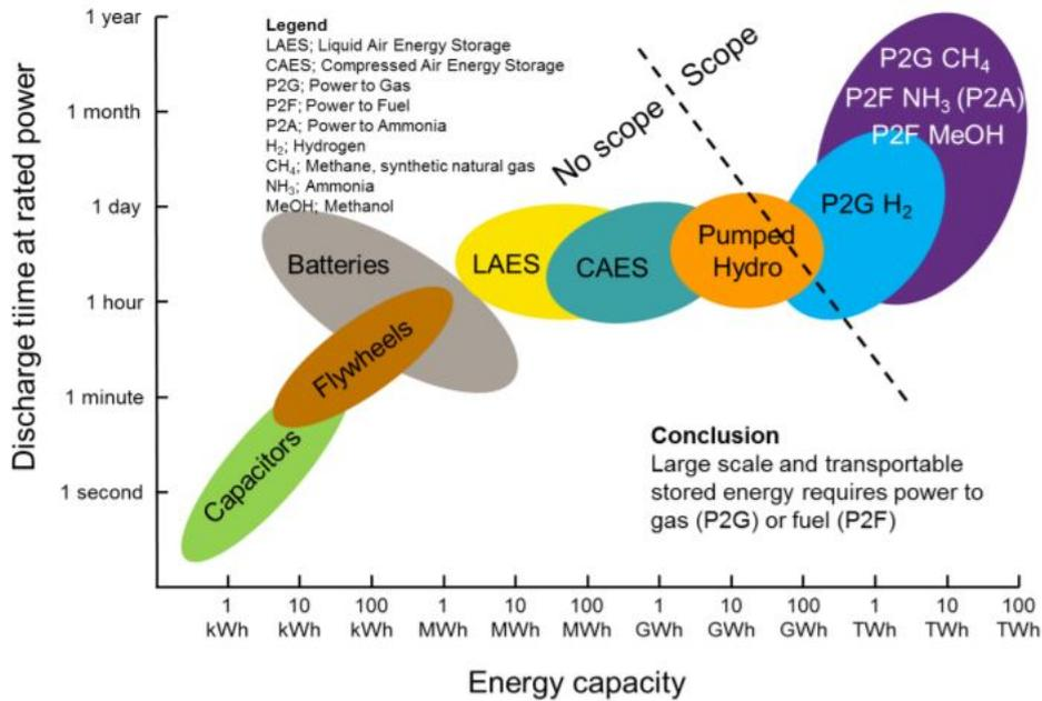
Figure 1.2: Discharge time versus the energy storage capacity of different energy storage techniques [7]
