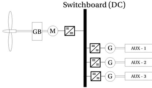
Figure 5.14: An electric powertrain configuration powered by an ICE with a direct current switchboard
