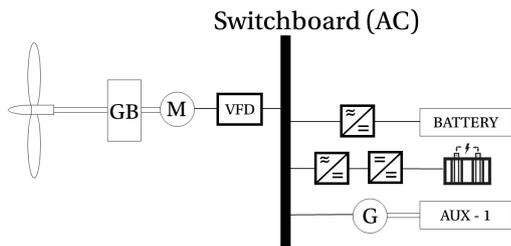
Figure 5.18: An electric powertrain configuration powered by an ICE, a battery and a fuel cell with an alternative current switchboard
