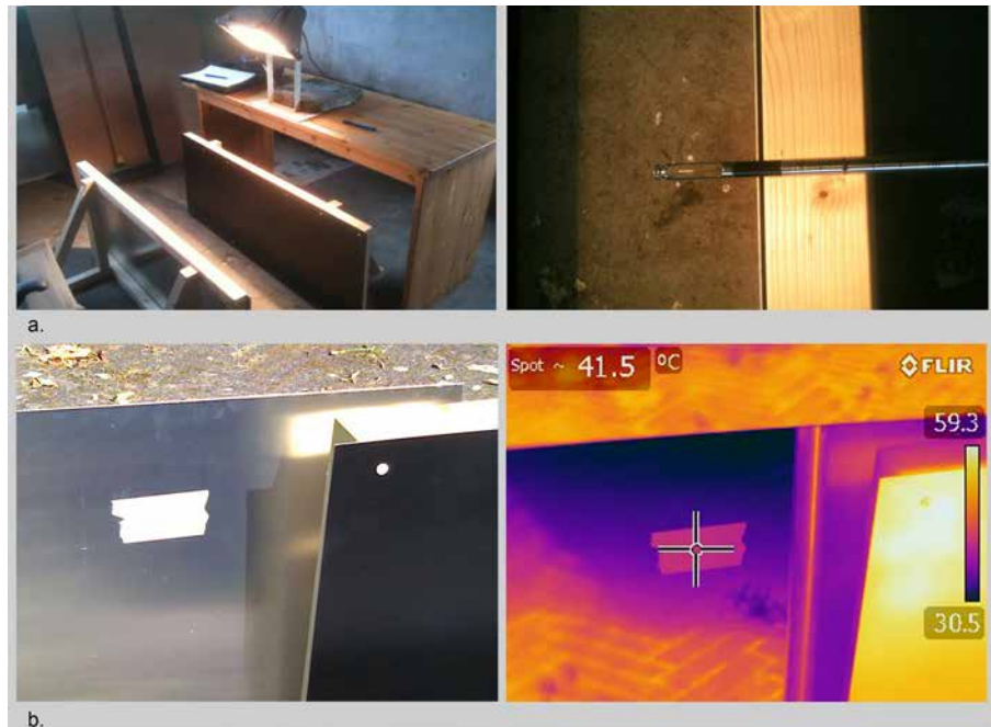
FIGURE 6.1 a. The indoor laboratory set (left) and the anemometer measuring the speed of the vertical air flow (right) (27-08-2013); b. The surface temperature of black coated aluminium and bare aluminium (left) measured with a thermal camera (right) (05-09-2013).
