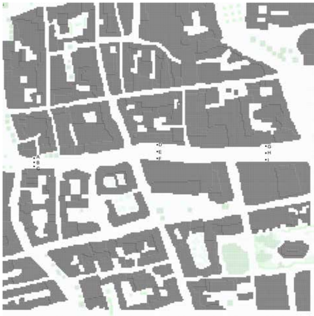
FIGURE 9.13 The model input in ENVI-met showing the Grotemarktstraat and surrounding in The Hague with receptor points A to I.
