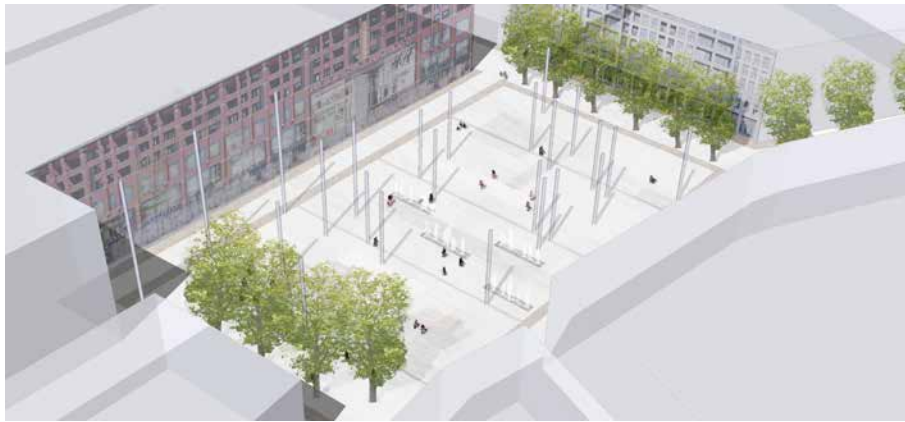
FIGURE 8.43 Vredenburgplein with ventilating solar chimneys by Vincent Peters, WUR.
