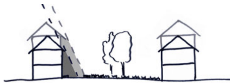
FIGURE 9.4 Sketch of solar angle ( 61.5^\circ ) on the 21 of June at noon with two or three building layers in section AA' in Fig 9.5.
