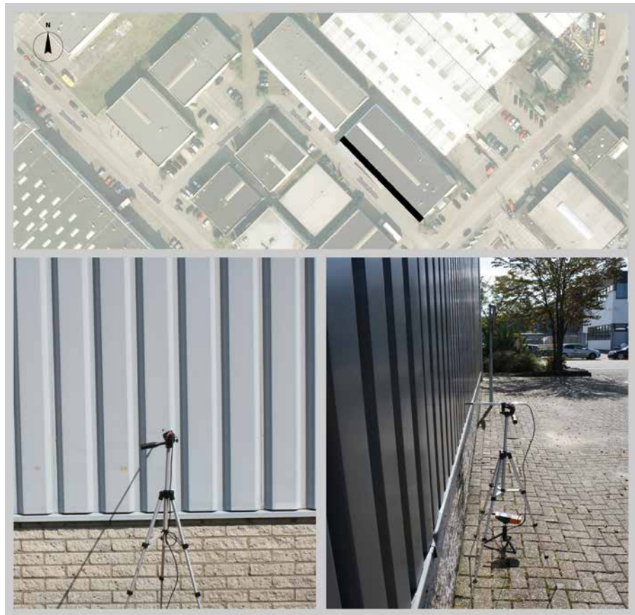
FIGURE 6.2 A map of the measurement location and images of the measurement setup at the white (left) and black (right) façade (27-08-2014).
