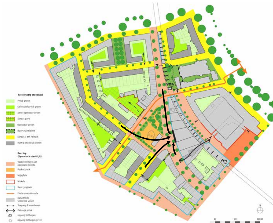
FIGURE 9.29 Expected thermal induced air currents with a dark façade drawn into the master plan Insulindeplein
