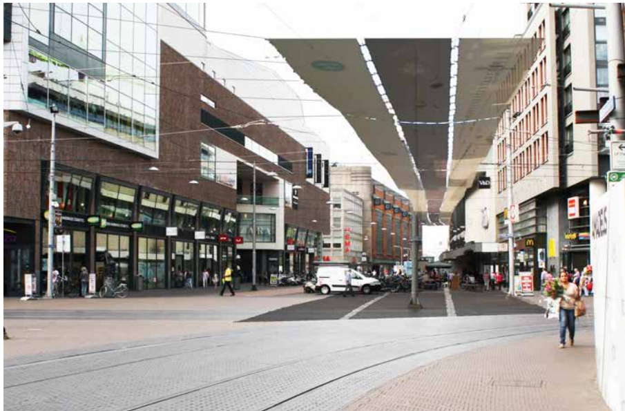
FIGURE 9.12 The Grotemarktstraat in The Hague with canvas sheets to improve thermal comfort on hot days.
