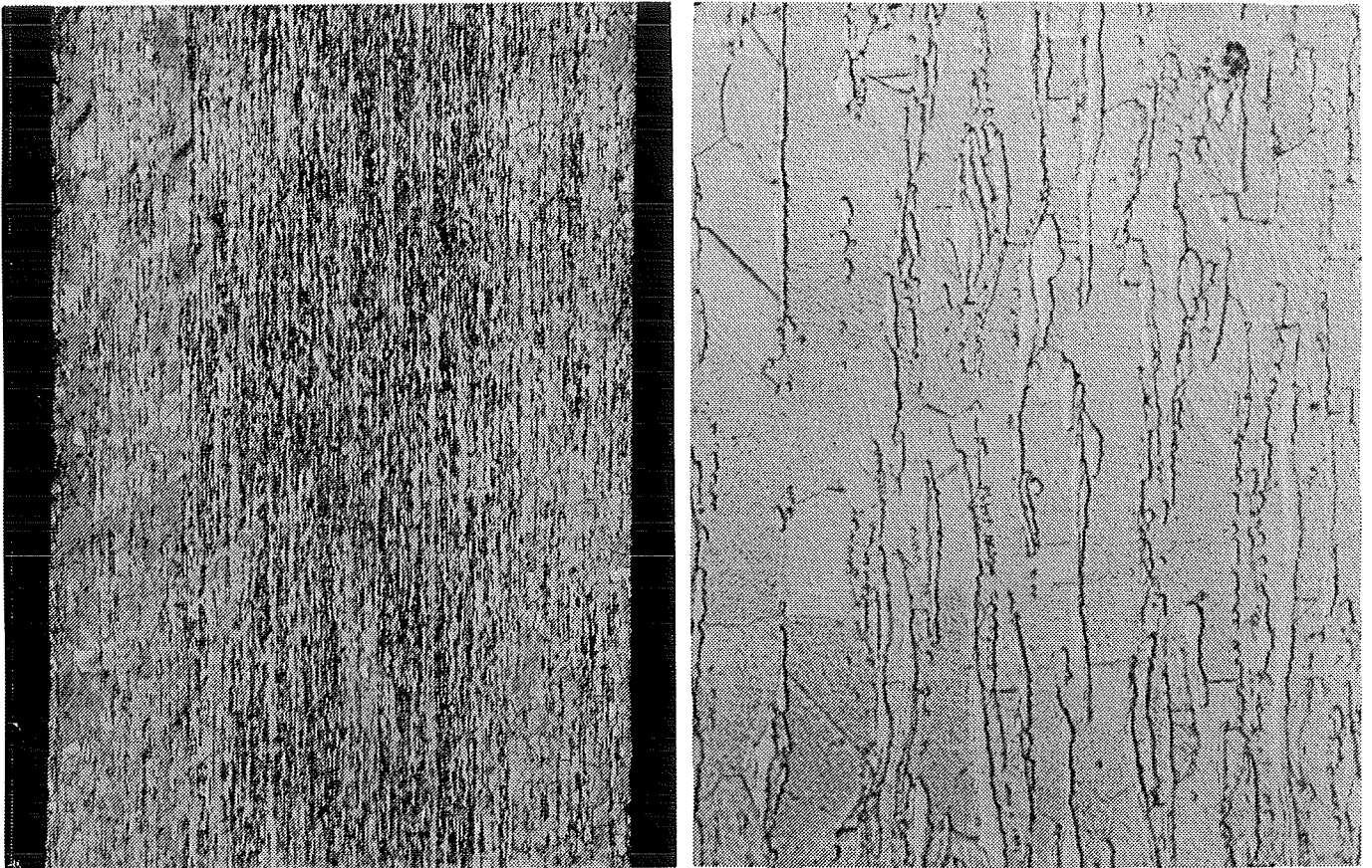
Figure 15. Microstructure photographs of AuPtRh 69/30 after rolling and homogenisation at 1100°C, left 100x BF, right 1000x BF OI.
