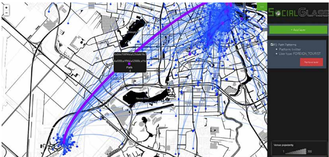
FIGURE 37 Origin-Destination (OD) paths. Larger edge thickness and color density illustrate larger flow volumes.
