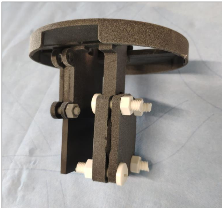
Figure 12: Image of the three 3D printed supports mounted together. The cathode support can be seen with a block of graphite on the left. The main support can be seen on top holding the two other supports together.
