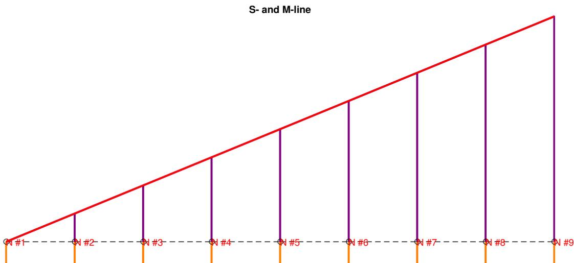
Figure 3.25: S- and M-distribution, cantilever beam, 8 linear elements
