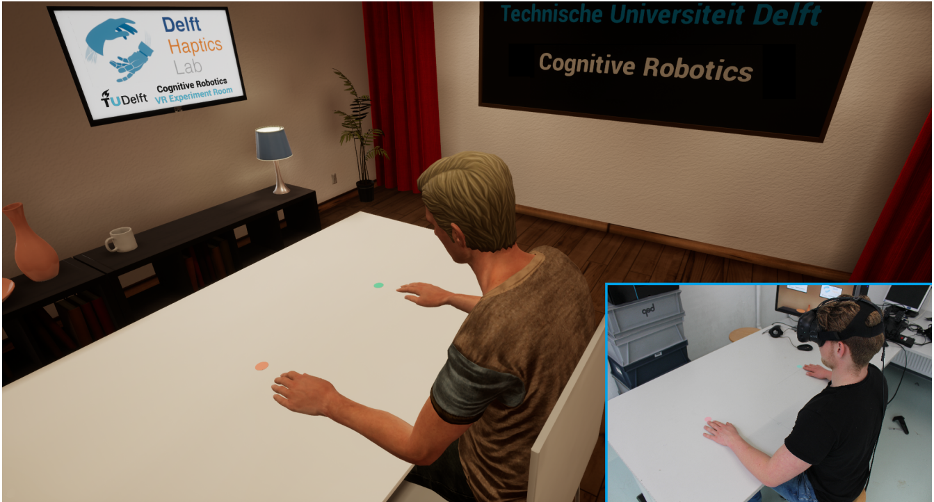
Fig. 2. The virtual environment for the static VRHI condition, with the participant in the actual experiment room in the bottom-right corner. The colored stickers placed on the table(s) represent reference points for the proprioceptive drift measurements and calibration purposes. The experiment leader sat on the opposing side of the table, and used a motion controller to stroke and tap the right hand of the participant, who received congruent visual feedback from the motion controller in VR.
