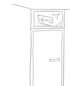
emergency exit light
