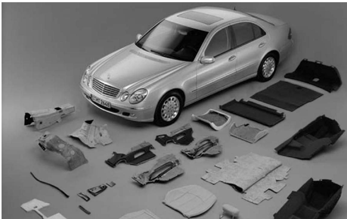
Figure 2.4 Flax, hemp, sisal, wool and other natural fibers are used to make interior Mercedes-Benz E-Class components. ([www.daimlerchrysler.com](http://www.daimlerchrysler.com))
