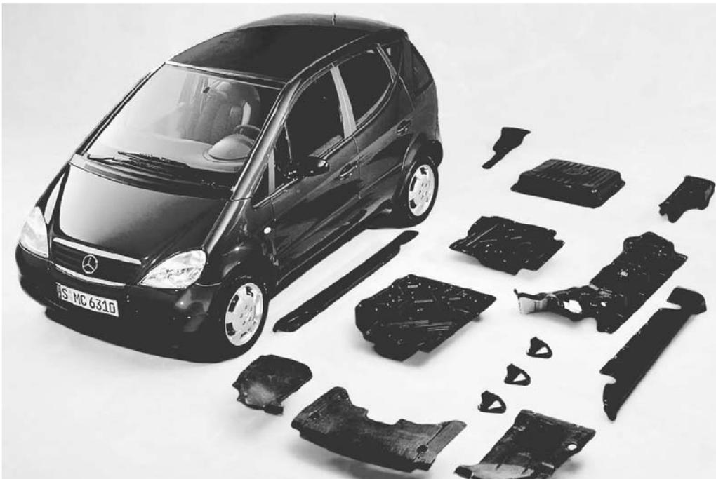
Figure 2.1 Parts made of glass mat thermoplastics (GMT) in Mercedes A-class. ([www.daimlerchrysler.com](http://www.daimlerchrysler.com)).
