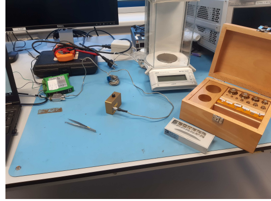
Figure 6.14: Measuring the sensor voltage output with the use of the weights.
