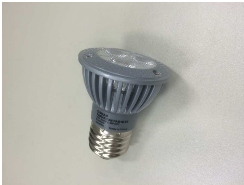
Fig 5-3 Load 1 – OSRAM 4.5 W LED lamp
