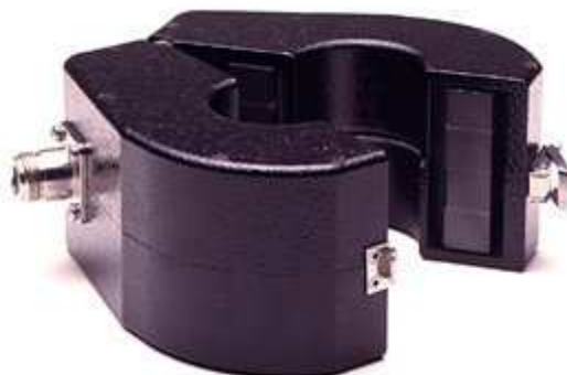
Fig 3-2 Current probe ETS 94430-5
