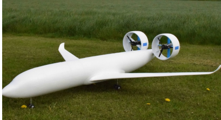
Figure 2.2: Delft University Unconventional Configuration - DUUC
