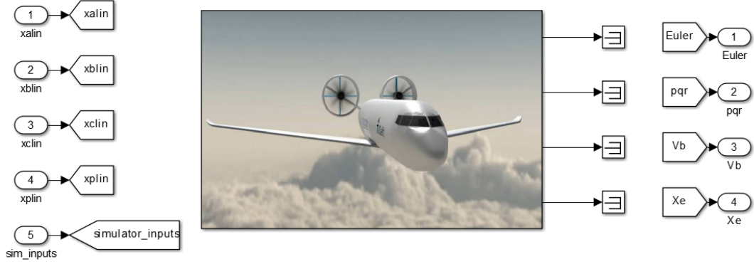
Figure 5.4: Top level structure of the flight mechanics model in PHALANX
