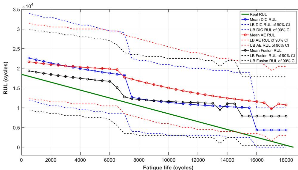
Fig. 14. Estimated mean RUL and 90% confidence intervals for specimen03.
