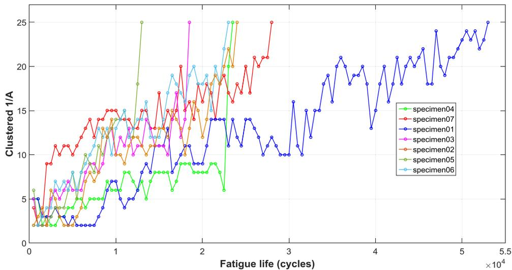
Fig. 10. Clustered AE degradation histories of seven open-hole specimens.
