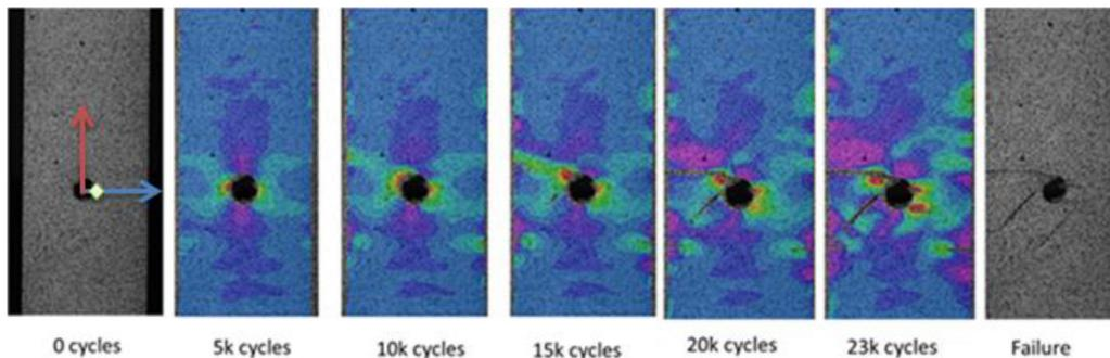
Fig. 4. Axial strain distribution of specimen02.
