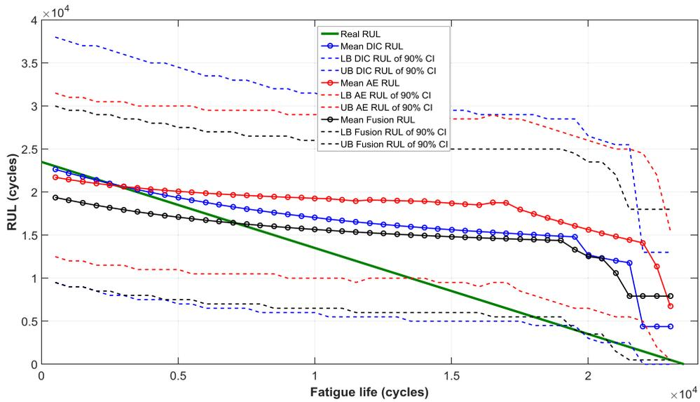
Fig. 15. Estimated mean RUL with 90% confidence intervals for specimen04.
