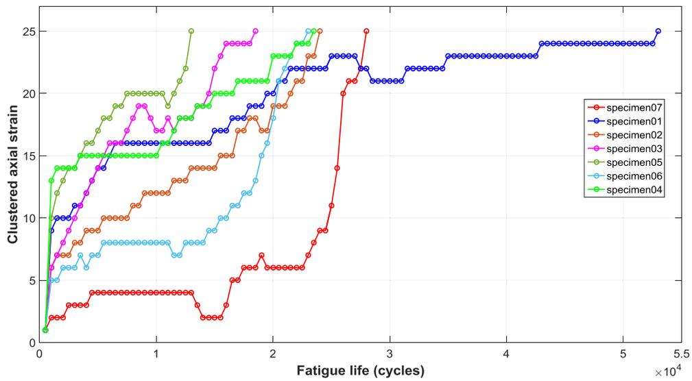
Fig. 7. Clustered axial strain degradation histories of seven open-hole specimens.
