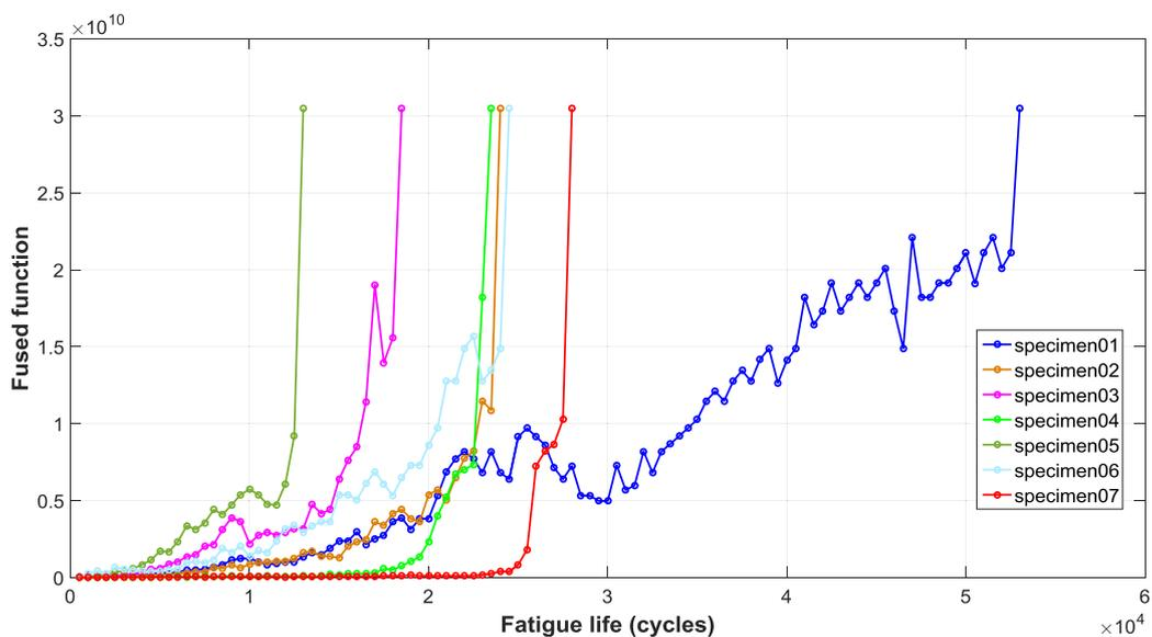
Fig. 12. Fused degradation histories of seven open-hole specimens.
