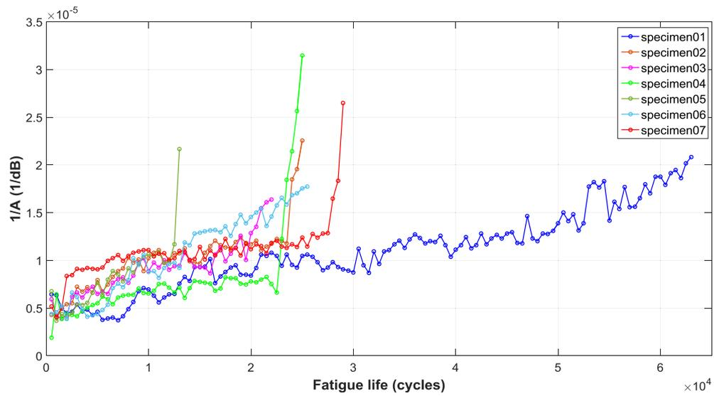
Fig. 8. AE degradation histories of seven open-hole specimens.
