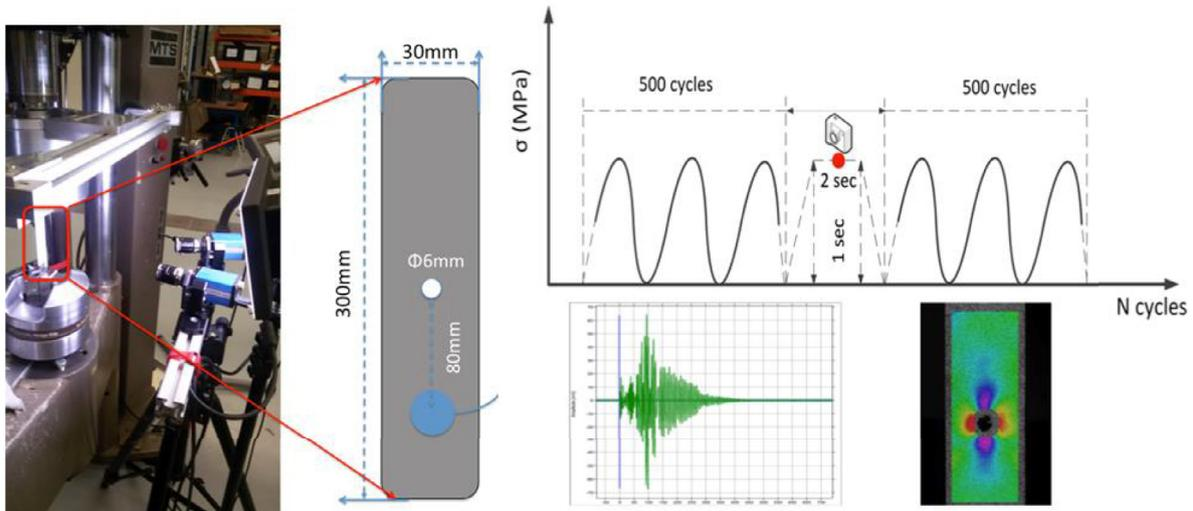
Fig. 3. The experimental set-up and the acquisition data process [37].
