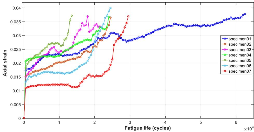
Fig. 5. Axial strain degradation histories of seven open-hole specimens.
