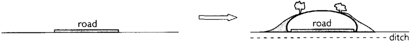
System 3b. A cover for roads and railway lines, extra costs 350 - 550 Euro
