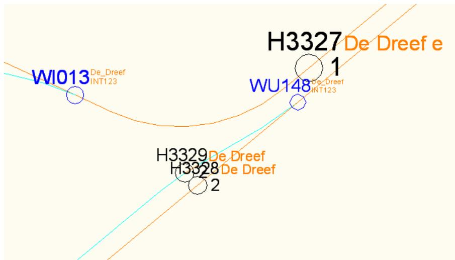
Figure C.3: End stop of the line with an extra “e” to its name
