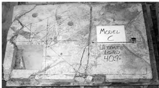
Figure 3.17: Specimen 3 after failure [3].
