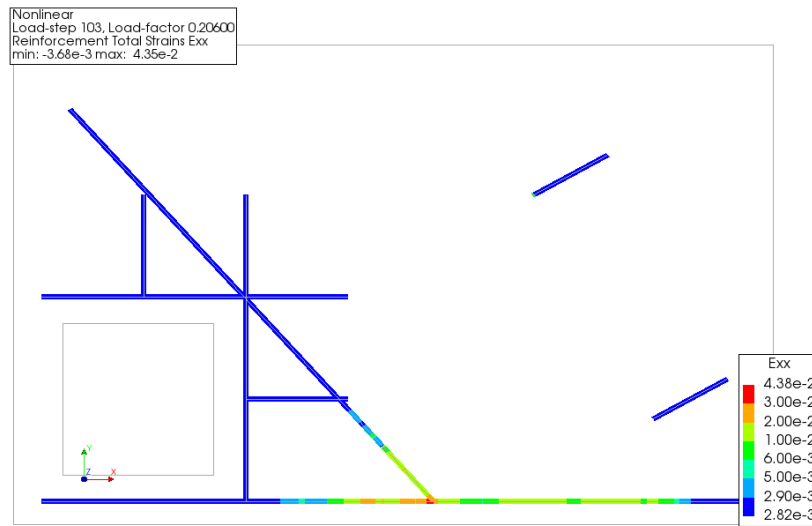
(b) Rebar strain (Exx) at specimen 4 TR model
