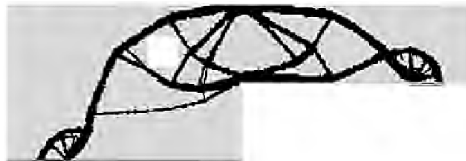
Figure 3.2: The optimal topology of a dapped beam with an opening according to full homogenization method [13].
