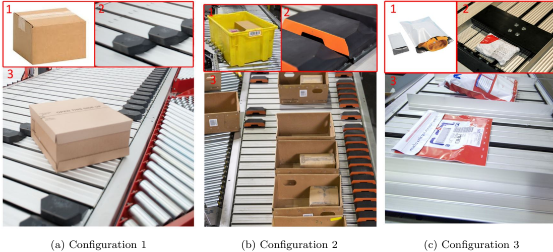
Figure 1.3: Current sorter designs (1: parcel type that can be handled on the system, 2: slider and carrier design, 3: an overview of sorter) [14]
