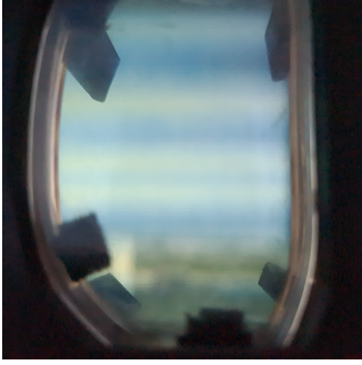
Figure 11: Example of the transmitter at seven centimeter sending data at 3000 symbols per second.
