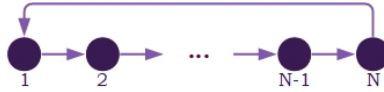
Figure 2.5: Using a graph representation for a finite discrete periodic time of length N .
