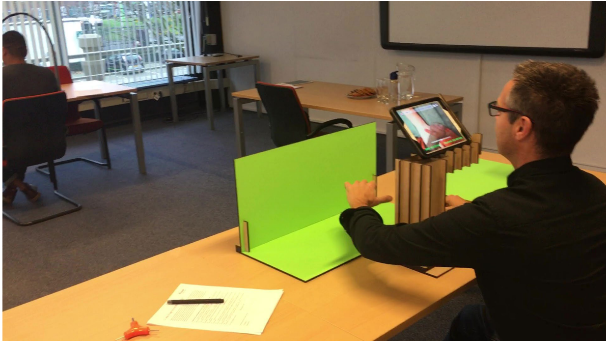
Figure 66: Hands have to be kept high up to get them in the work area
