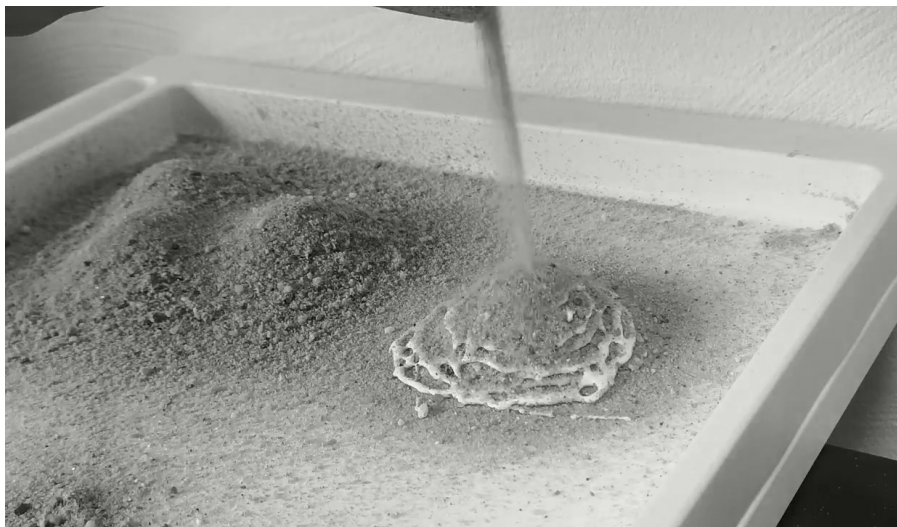
Material- Sand/ Clay/Silt Binder- Wood Glue
