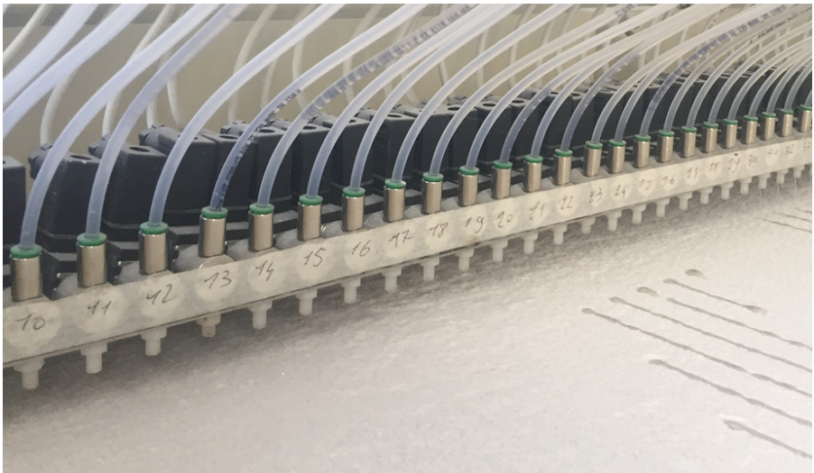
Technique: HI-Tech/ Binder Jetting Technology Material: Sand/Magnesia based cement Binder: Saline Water Solution
