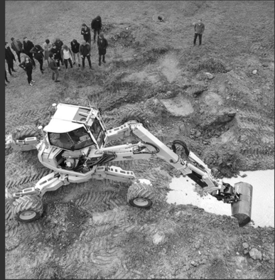
[HEAP-ETH Zurich, Prototype Autonomous Digger]
