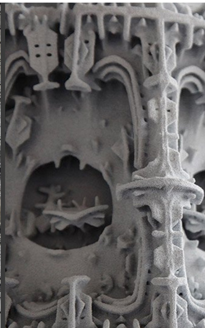
Michael Hansmeyer's Digital Grotesque detailed wall element using the powder bed production technology.
