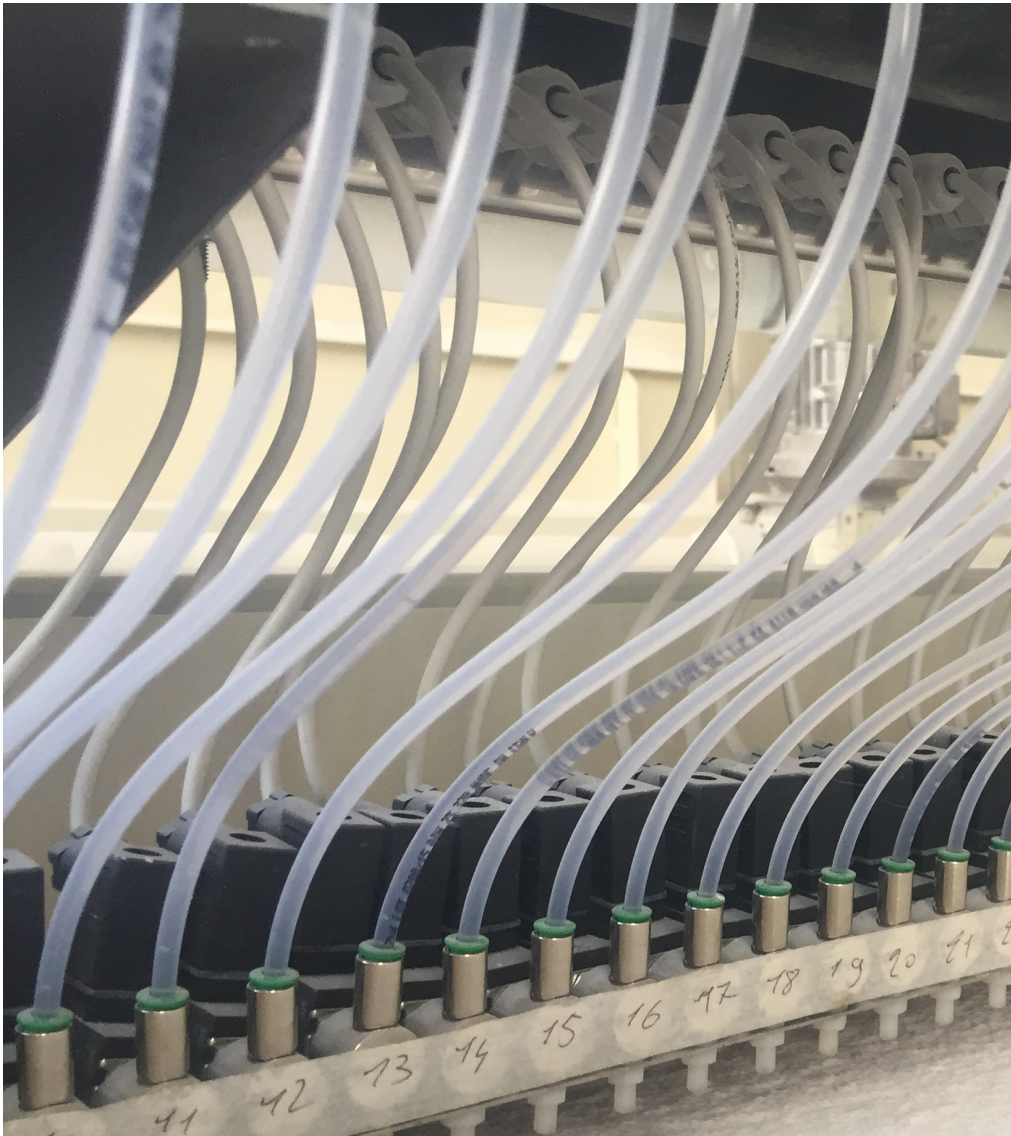
Process of alternating layers of granular material and ‘writing’ on them with a binder that turns the granular material into a shape.
