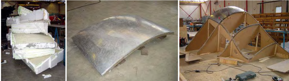
Fig. 8-10. Left over polystyrene moulds used to make negative concrete moulds (left), exploformed aluminium panel (center) and fitting of a panel on a wooden fitting mould (right).
