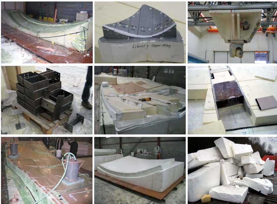
Fig. 19-27. Milling machine at Marin (19), scale model of upper wing of 'The Library' (20) and production of the roof segments at Holland Composites (22-28). Vacuum injection of the top layer on foam block milled by Marin (21). Insert to be placed in the GRP sandwich roofs in order to make a connection between the roofs and the columns (24). Placement of foam blocks and glass fibre matts, which will become stringers (23). Vacuum injection of the bottom layer (25). Final result, in this case an early prototype (26). Discarded foam moulds (27).
