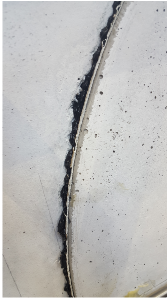
(a) Extrusion of bitumen (test 2a ULS)
