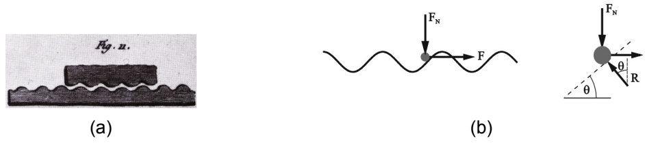
Figure 2.17: Interaction between the surface roughnesses between two bodies, [14]
