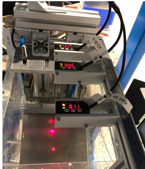
Figure 3.17: Positioning of the lasers distance sensors in the setup for measuring the plate deflection upon wave impact.
