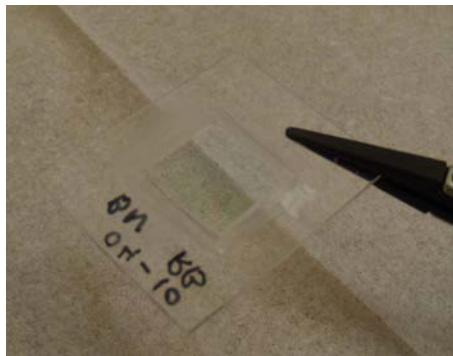
Figure 3.8: Picture of hBN on PMMA suspended in the plastic window after removing the Si-wafer.
