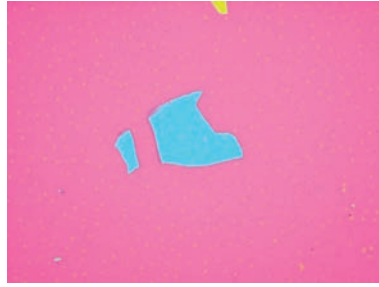
Figure 3.5: A suitable hBN flake on a chip covered with PMMA.
