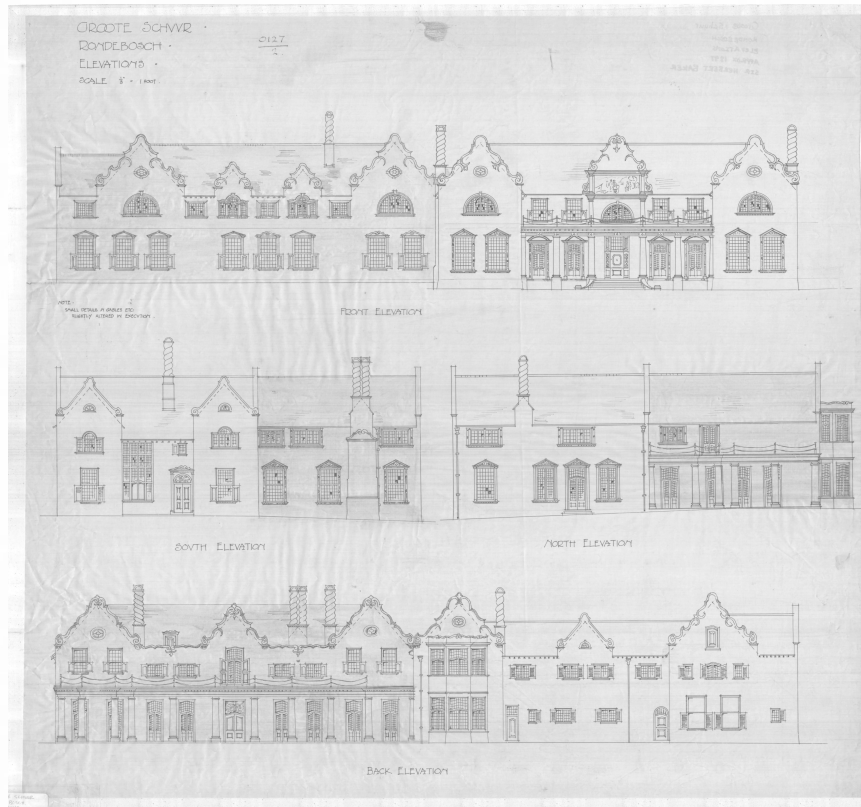
Figure 13 - Sir Herbert Baker's elevations for the renovation of Groote Schuur, showcasing quintessential Cape Dutch details.
