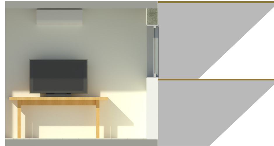
Figure 90: Section view of the exterior shading strategies over both window and walls (2.0 m overhang) of Room 38, considering an external support (green). Source: Own
