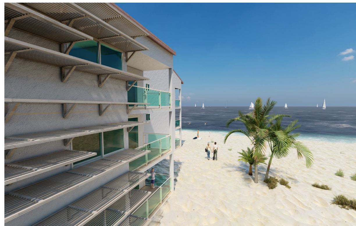
Figure 99: Application of Shading Overhangs of 1.0m in length. Source: Own.
