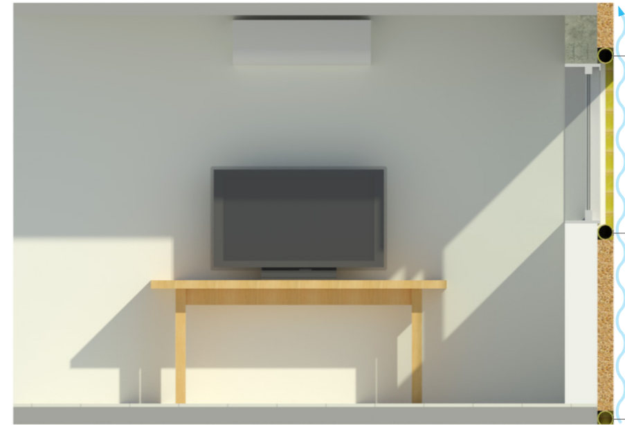
Figure 94: Section view of the ventilated sustainable facade layers added to the existing walls on Room 9. Source: Own
