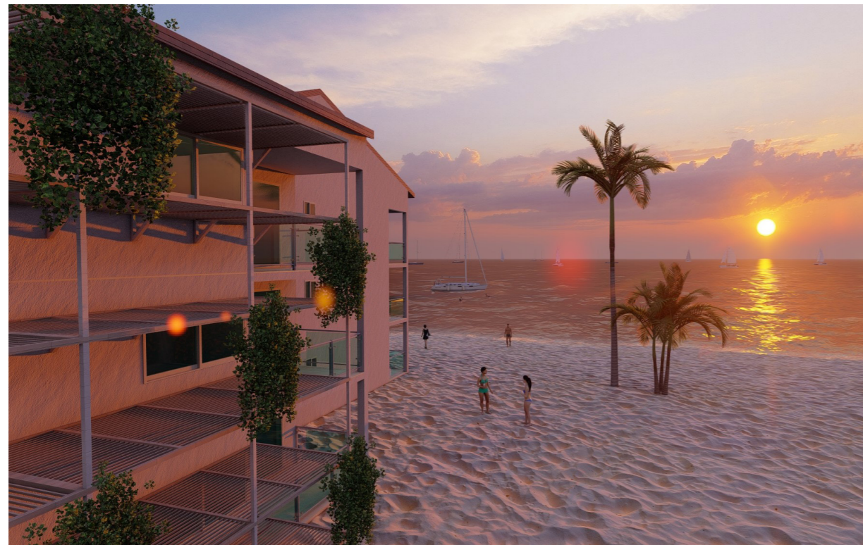
Figure 101: Application of Shading Overhangs of 2.0m in length. Source: Own.
