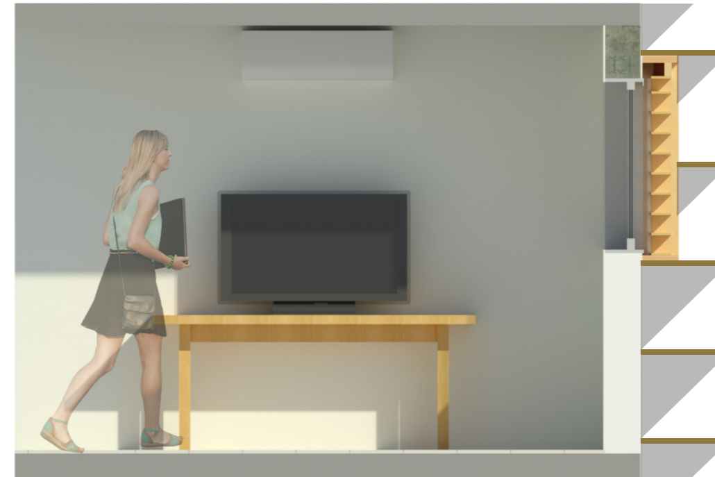
Figure 87: Section view of the exterior shading strategies on both window and walls. Source: Own
