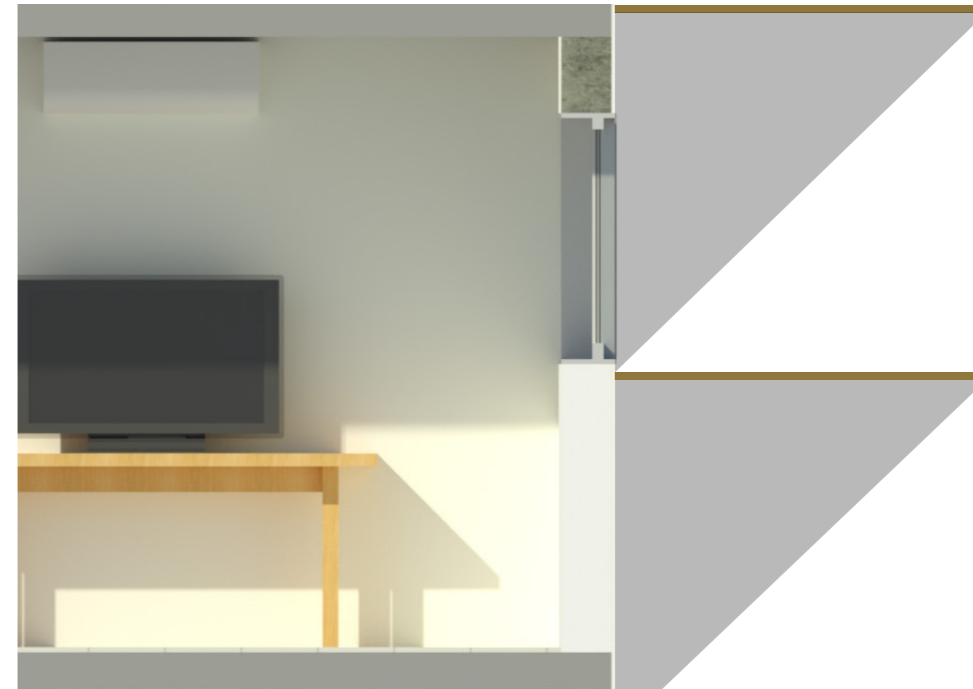
Figure 89: Section view of the exterior shading strategies over both window and walls (1.5 m overhang) of Room 38, considering an external support (green). Source: Own
