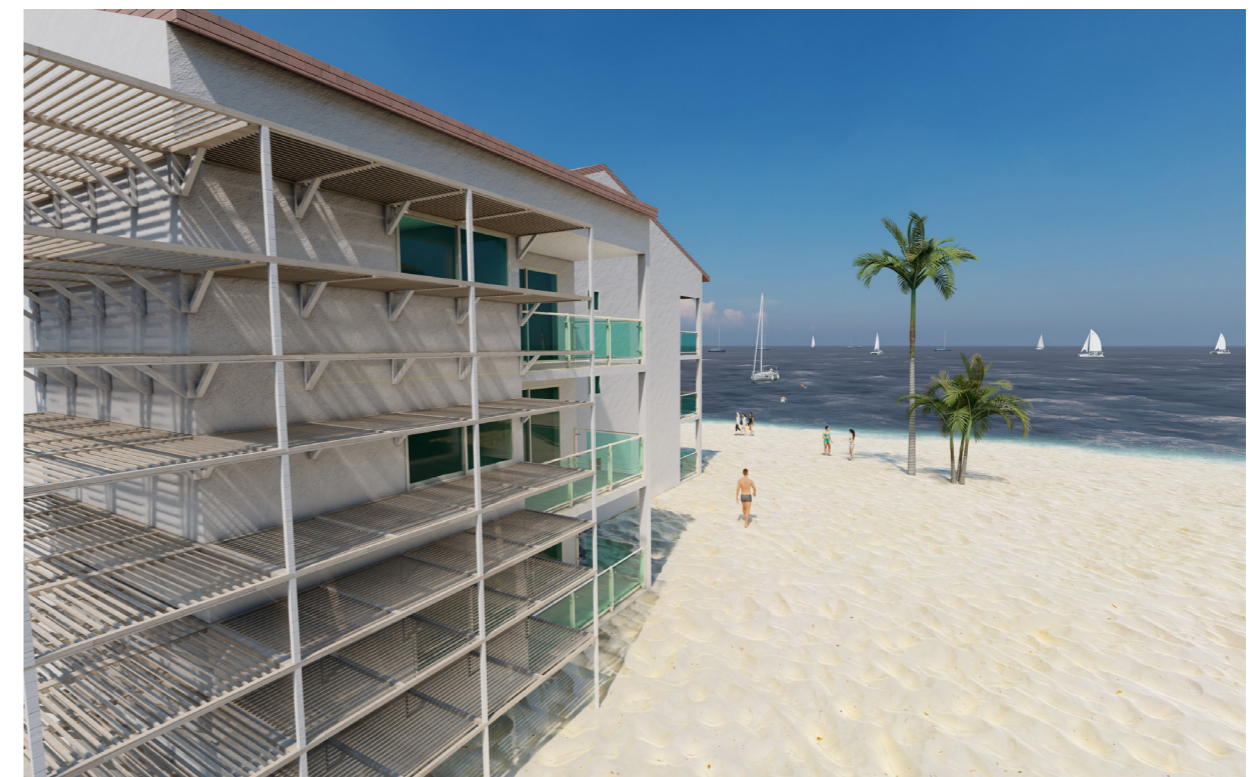
Figure 100: Application of Shading Overhangs of 1.5m in length. Source: Own.
