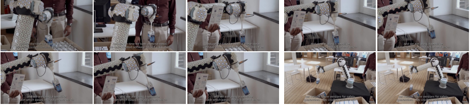
Figure 4.7: Collision avoidance task - Illustration of a successful alternate path generation behavior. L to R top row: After the robot has picked up an object, an obstacle is introduced along the robot trajectory to the object drop off location. L to R bottom row: The SoT controller computes an alternative path avoiding the obstacle while respecting the collision avoidance constraint and the trajectory execution task is successfully completed thereafter.
