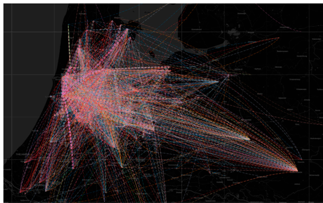
Figure 2. Example of an activity-based spatial material flow analysis (AS-MFA) result, concerning construction and demolition waste (CDW) originating in the Amsterdam metropolitan area (AMA), in tons/year, from origin (disposal location) to destination (storage or treatment location). Each color represents a CDW category.
