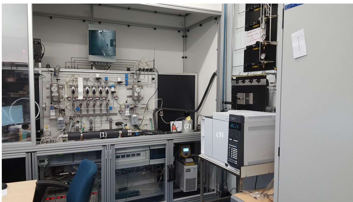
Figure B.1: Overview of the experimental system: (1) LED-based annular photoreactor; (2) Verborg reactor; (3) gas chromatograph
