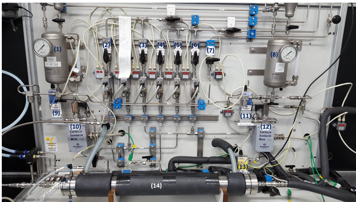
Figure B.2: Experimental system: (1) Toluene vessel; (2) Oxygen dilution line MFC-12; (3) Oxygen to CEM-2 MFC-16; (4) Nitrogen dilution line MFC-14; (5) Nitrogen to CEM-2 MFC-13; (6) Nitrogen to CEM-1 MFC-12; (7) Compressed air; (8) Water vessel; (9) Toluene MFC-18; (10) CEM-2; (11) Water MFC-11; (12) CEM-1; (13) Pressure meter; (14) LED-based annular photoreactor
