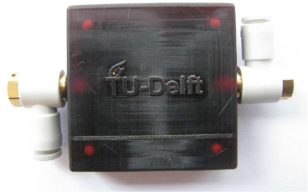
Figure 37: Final model of the encapsulation module, designed in SolidWorks. The module was fabricated in EWI at TU-Delft.
