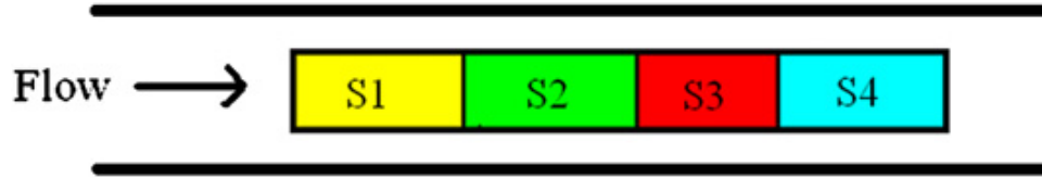
Figure 12: A flow insensitive TCD using several TCD regions [31].
