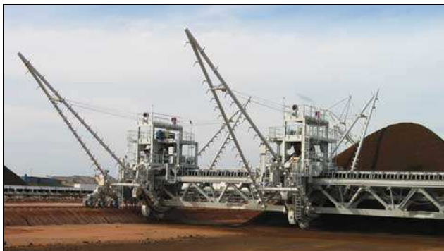
Figuur 2.6a: bridge type bucket wheel reclaimer
