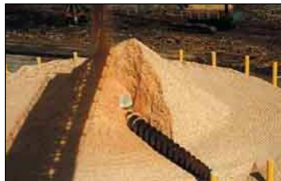
Figuur 2.8b: rotary screw reclaimer
