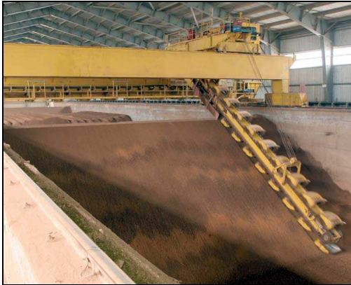
Figuur 2.5a: bridge type bucket wheel reclaimer
