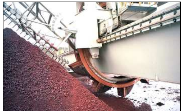
Figuur 2.6b: bucket wheel
