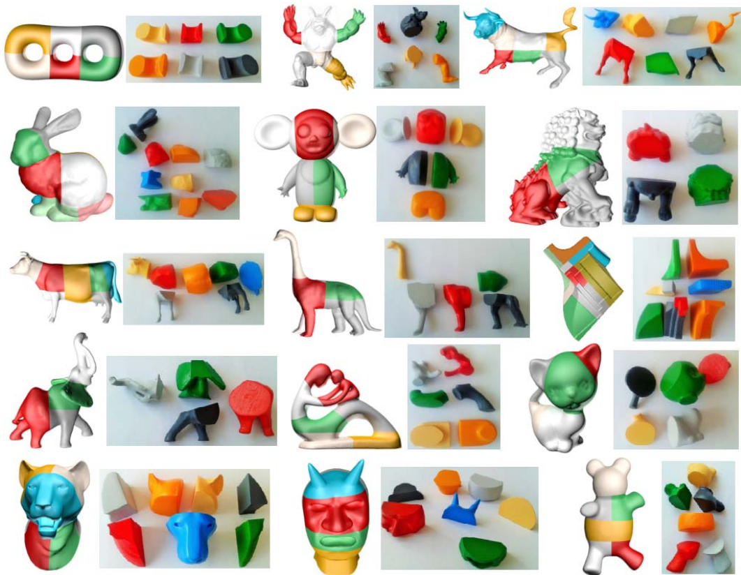
Figure 7. Some partitioning results by users with a few interactions using our proposed tool. For each model, the user's partitioning result and its printed parts are shown. The model volumes are 3Holes (8066.9cm 3 ), Armadillo (2288.82cm 3 ), Bull (2281.62cm 3 ), Bunny (6003.38cm 3 ), Cheburashka (3288.39cm 3 ), Chinese_Lion (6001.62cm 3 ), Cow (3277.76cm 3 ), Dinosaur (1299.09cm 3 ), Elephant (2232.42cm 3 ), FanDisk (5726.12cm 3 ), Fertility (3195.51cm 3 ), Kitten (6581.03cm 3 ), LionHead (4257.72cm 3 ), Monster (7330.87cm 3 ), Toy (4594.35cm 3 ), and the printer volume is 18.0cm × 17.0cm × 16.0cm.
