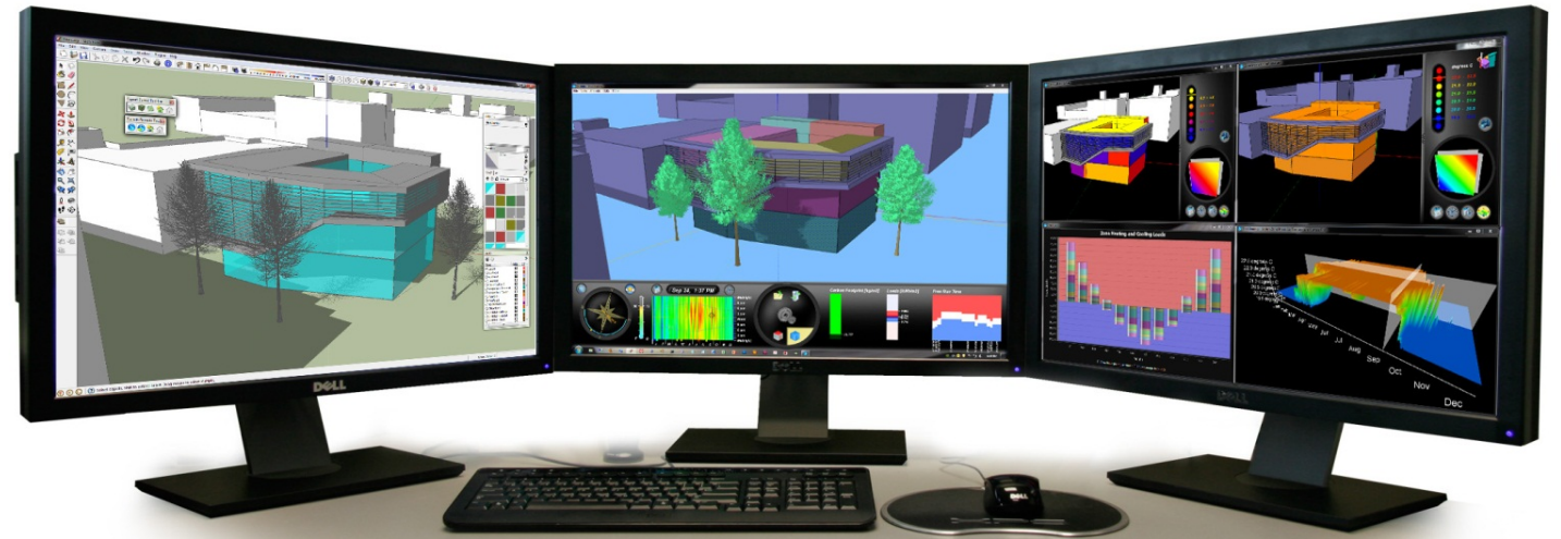
The workstation's left screen shows the CAD input, while the center shows the translated model, and the right contains BES output. (Pratt et al. 2012)
