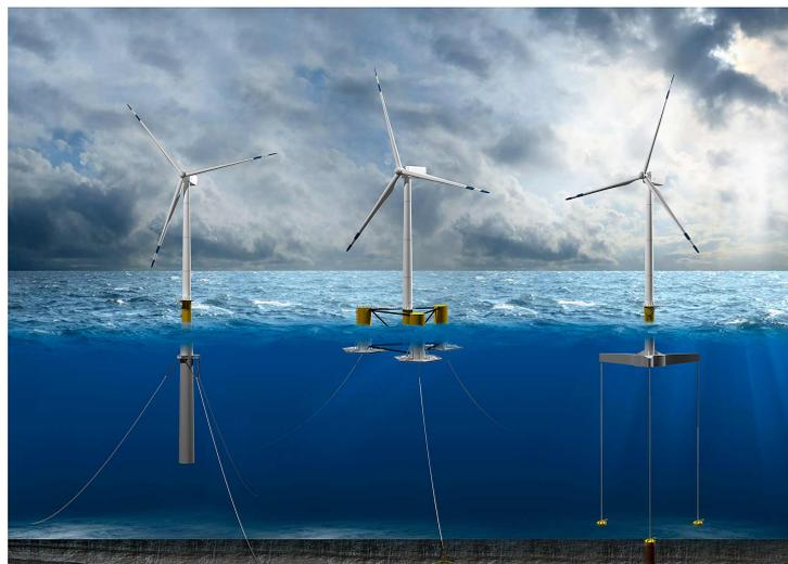
Figure 2.4: Types of floaters used for FOWT. Left: Spar buoy. Middle: Semi-submersible platform. Right: Tension-leg platform. Source:[42].
