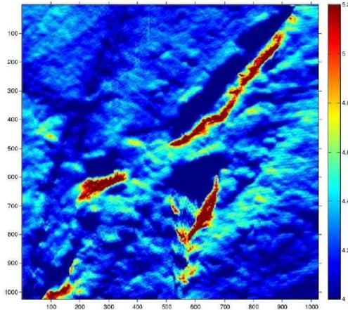
**Figure 1.** Atom-force microscope image of a small region of the surface of a vibrating NbTi wire used by Rich Haley and Chris Lawson (Lancaster University) to generate superfluid turbulence, as measured by atom-force microscope. The region extends  $1 \mu\text{m}$  in both  $x$  and  $y$  directions; the maximum height of the surface is  $16.1 \text{ nm}$  in the  $z$  direction.
