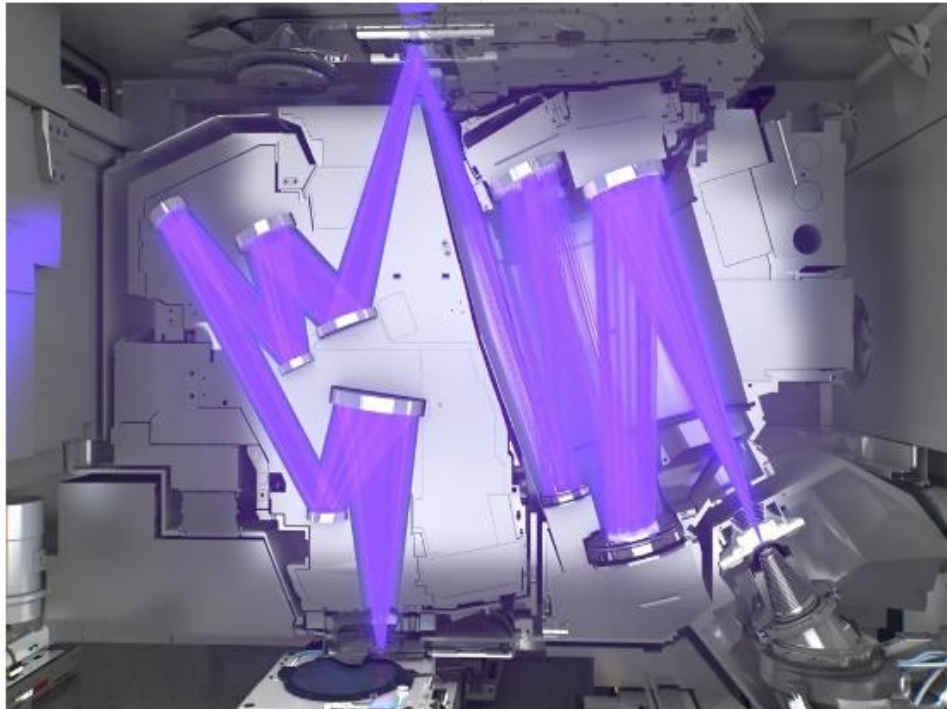
Figure 5 Lithography in EUV machine [1]
