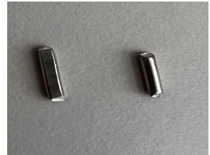
Figure 25 Tin sample after and before plastic deformation
