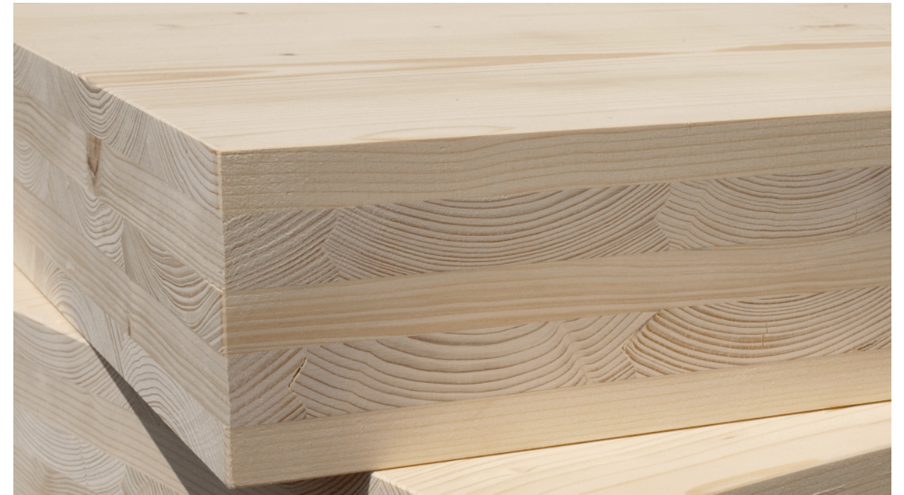
Fig 3.2.8.: Layered solid CLT panel with each layer being perpendicular the neighbouring ones. (CLT- Woodteq Houtconstructies, 2022)
