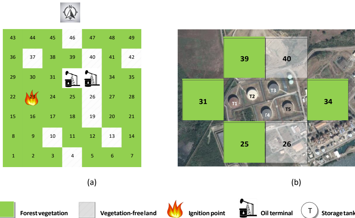
Figure 7. (a) Modeling the wildland-industrial interface as a lattice. Green cells are those with forest vegetation. The hatched cells are vegetation-free land. Cell 23 is where the ignition occurs. Cells 32
