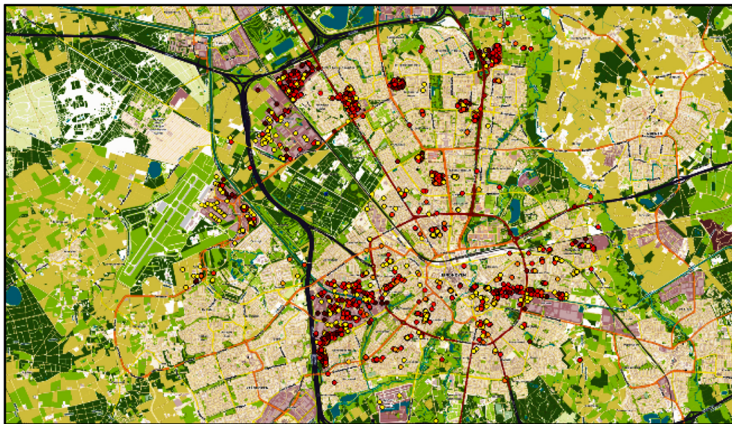
Fig. 7. Visual representations of the correlation between annual electricity usage of the industrial buildings and URBANIZATION-DEGREE ; the dots are representing the industrial buildings in and around the city, the colour spectrum from yellow (low) to red (high) depicts the annual electricity usage of the industrial buildings. (For interpretation of the references to colour in this figure legend, the reader is referred to the Web version of this article.)
